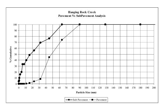
Figure 7.1 Pavement / Subpavement Analysis for Hanging Rock Creek.
