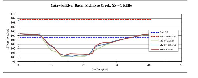
\* Note: Cross Section was established after repairs conducted at the Site.
