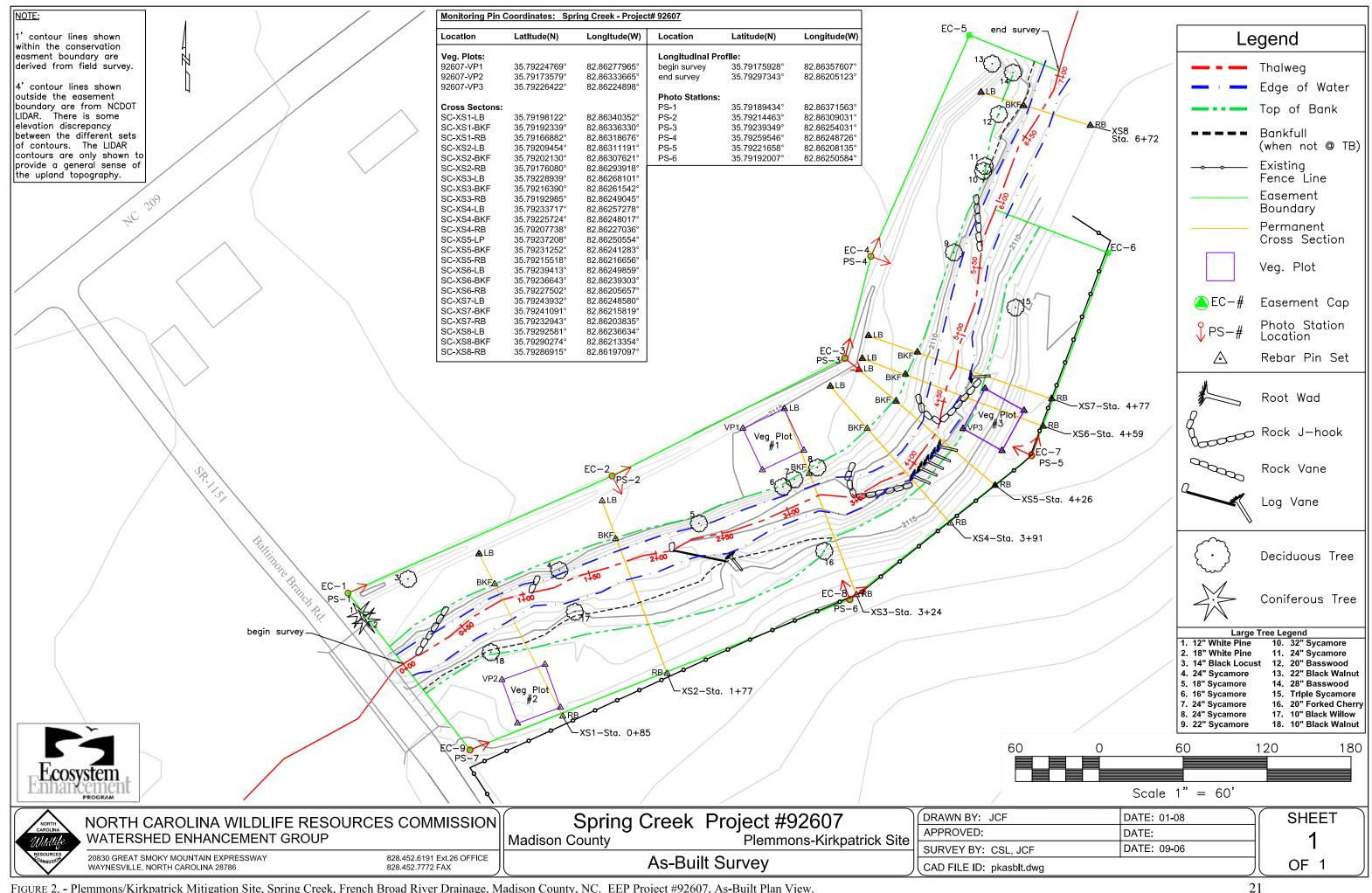
FIGURE 2. - Plemmons/Kirkpatrick Mitigation Site, Spring Creek, French Broad River Drainage, Madison County, NC. EEP Project #92607, As-Built Plan View.
