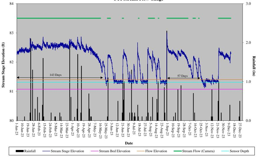
Rough Horn Swamp Restoration Site Hydrograph UT2 Stream Flow Gauge
