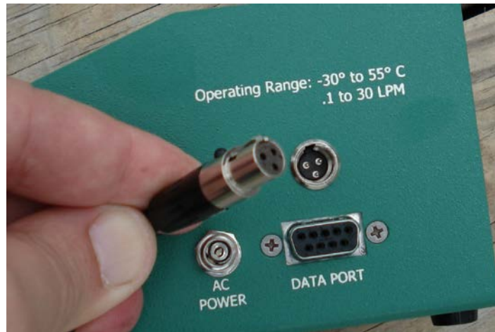
Figure 5. Temperature Probe Cable and Port.
