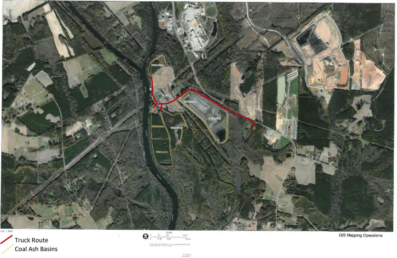
Figure 9. Onsite traffic patterns for trucks moving the ash from the basins to the proposed new beneficiation plant (provided by Duke Energy).
