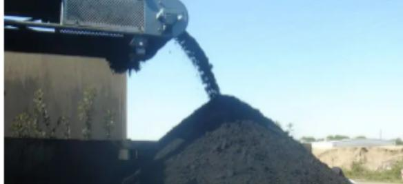
Pugmills are used in landfills to dry [waste sludges](#) by adding drying agents in the mixer so that the dried sludge can be landfilled. Pugmills are also used to stabilize waste dust such as fly ash, bed ash, and cement kiln dust. Newer applications include using pugmills to dry drilling fluids from the oil and gas industries, tunnel boring machines, and liquids from hydro excavation.
