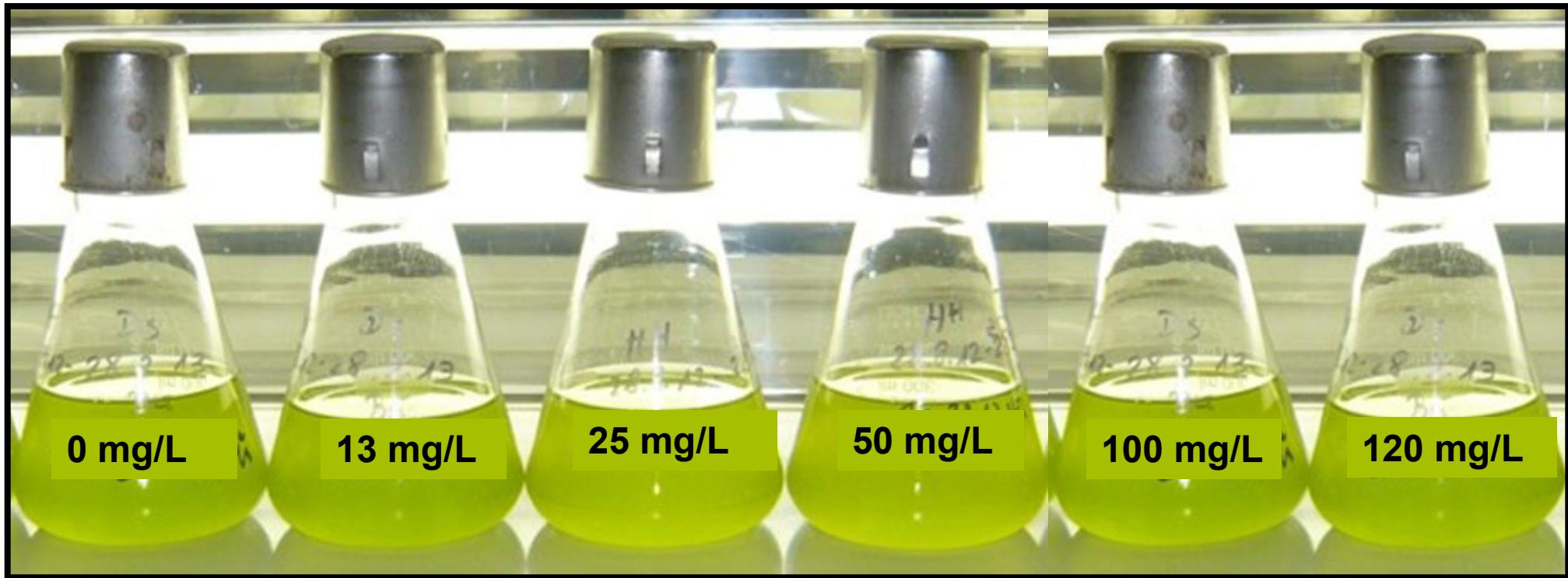
Measures inhibition of growth compared to 0mg/L Control
