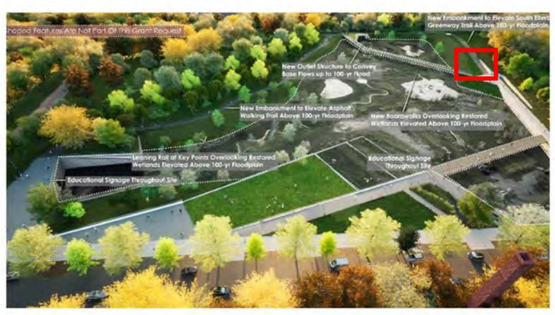
**New Outlet Structure with Complex Weir
