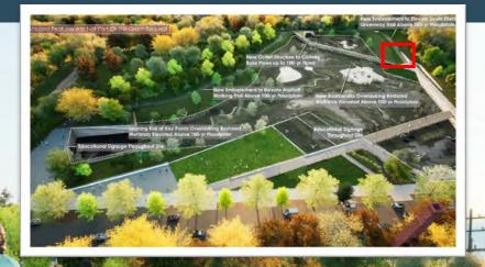
New Outlet Structure with Complex Weir Reduces Peak Flows Downstream by 34% During 100-yr Flood
