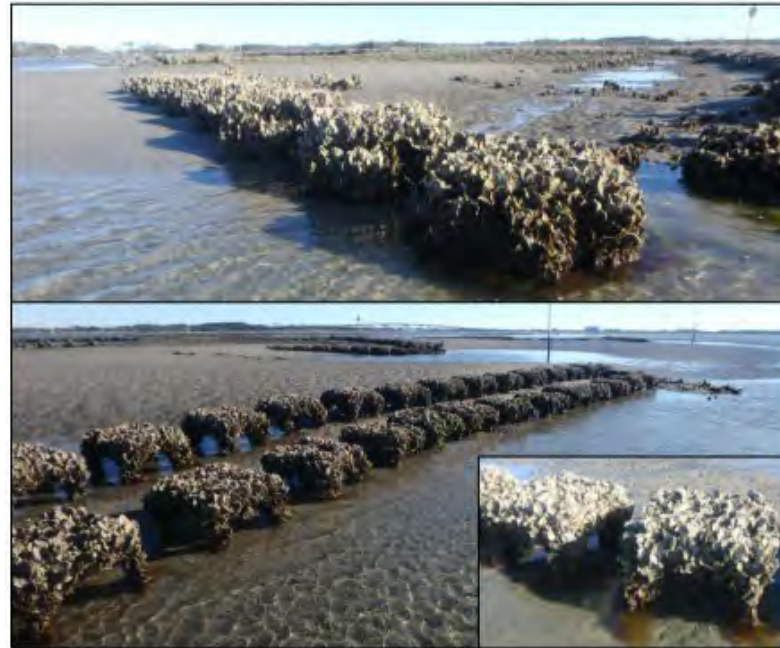
Figure 10. Examples of oyster growth on stacked Oyster Catcher™ Tables (top; 2 tables each stack); rows of single Oyster Catcher™ Tables (bottom) and close-up of oyster growth on Tables (bottom insert) 18 months after deployment in North Carolina.
