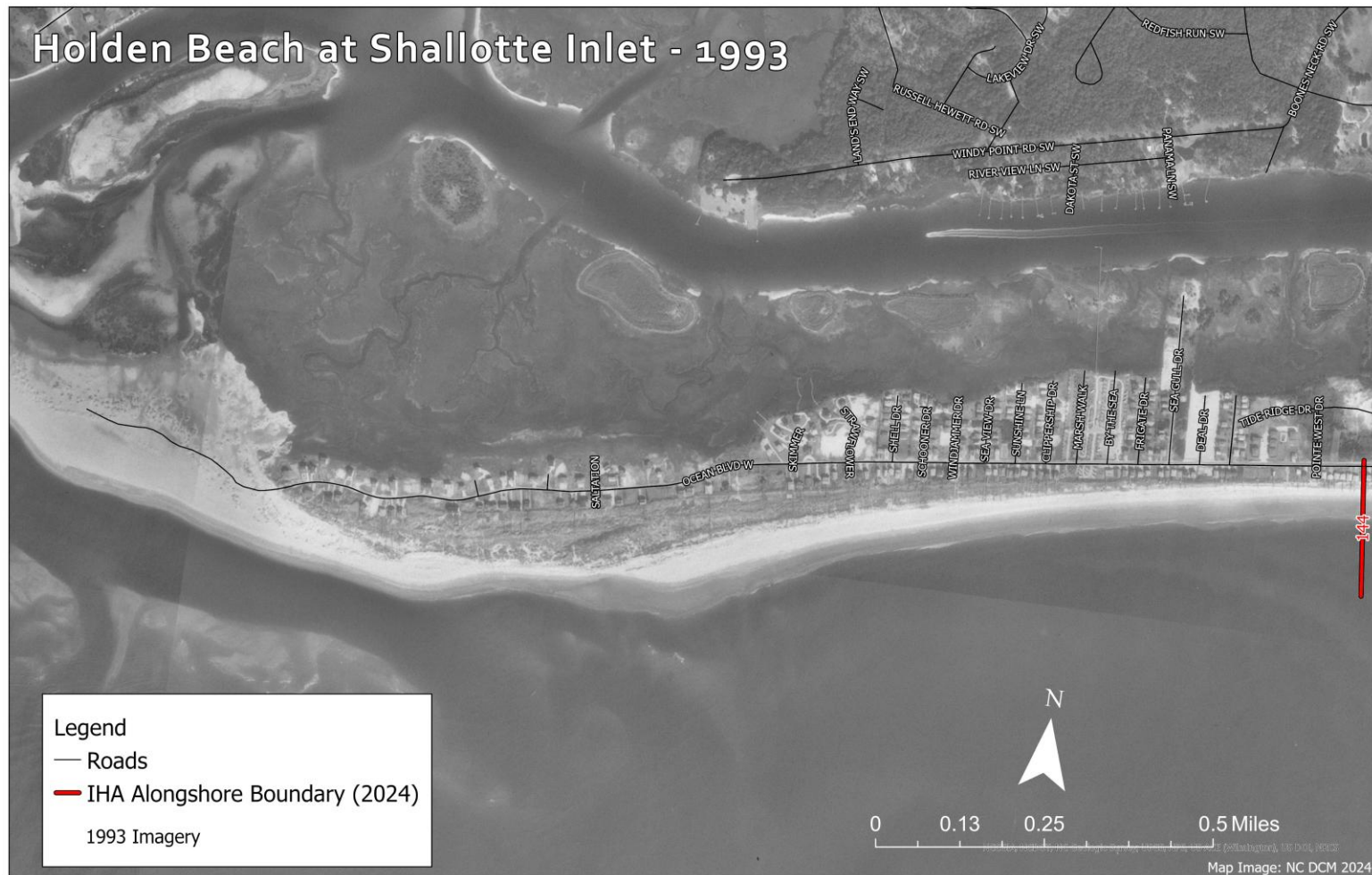
Figure D26. Shallotte Inlet at Holden Beach in 1993, shown relative to the 2024-2025 alongshore IHA boundary limit at transect 144 (marked by the red line on the right edge of the image). Although the prominent accretion area is less noticeable due to short-term erosion and the growth of vegetation, the ebb channel along the shoreline remains visible. Additionally, gradual longshore accretion toward the alongshore IHA boundary is still occurring, indicating ongoing shoreline changes in this dynamic environment.
