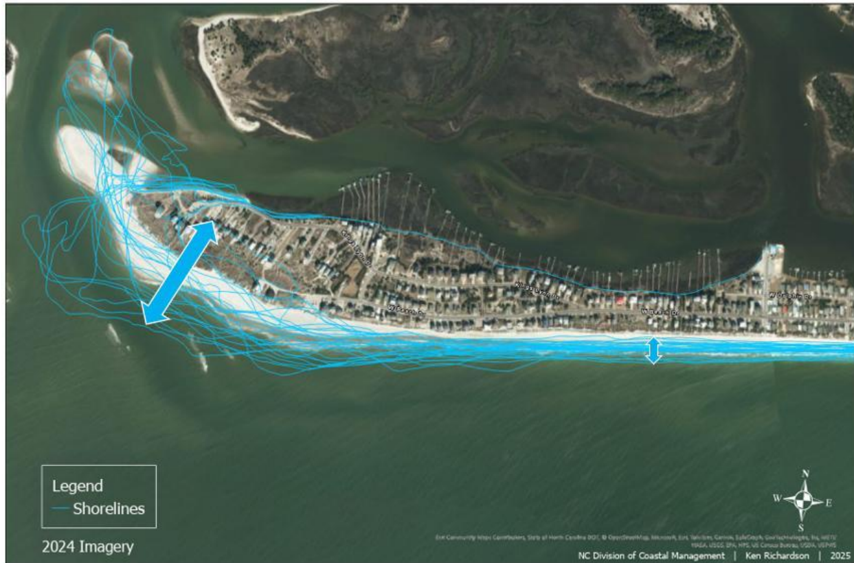
Figure 8. This map highlights the greater variability in shoreline position near inlets compared to farther away.
