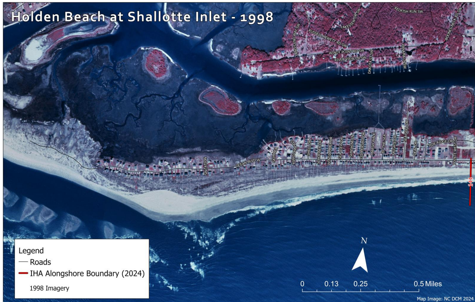
Figure D27. Shallotte Inlet at Holden Beach in 1998, shown relative to the 2024-2025 alongshore IHA boundary limit at transect 144 (marked by the red line on the right edge of the image), shows significant accretion. Here, the prominent accretion area is more noticeable as the ebb channel continues to remain along the shoreline. Additionally, gradual longshore accretion toward the alongshore IHA boundary is still occurring, indicating ongoing shoreline changes in this dynamic environment without any influences of beach nourishment.
