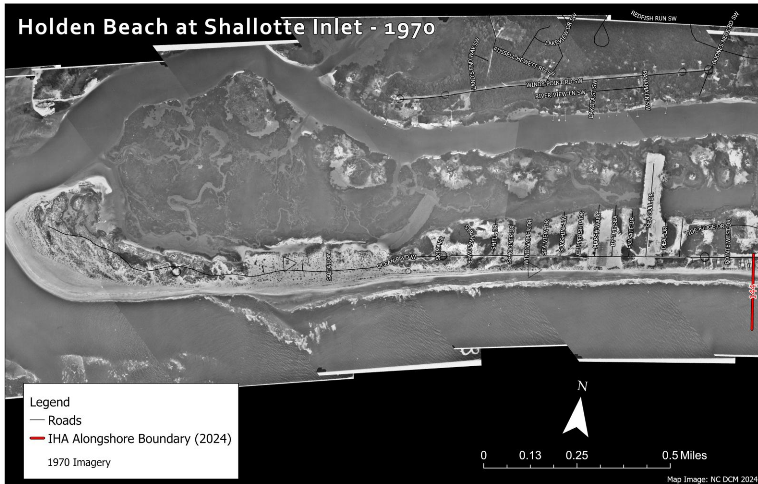
Figure D23. Shallotte Inlet at Holden Beach in 1970, shown relative to the 2024-2025 alongshore IHA boundary limit at transect 144 (marked by the red line on the right edge of the image). Shoaling along the oceanfront can be observed and is caused by inlet's ebb channel orientation along the shoreline.
