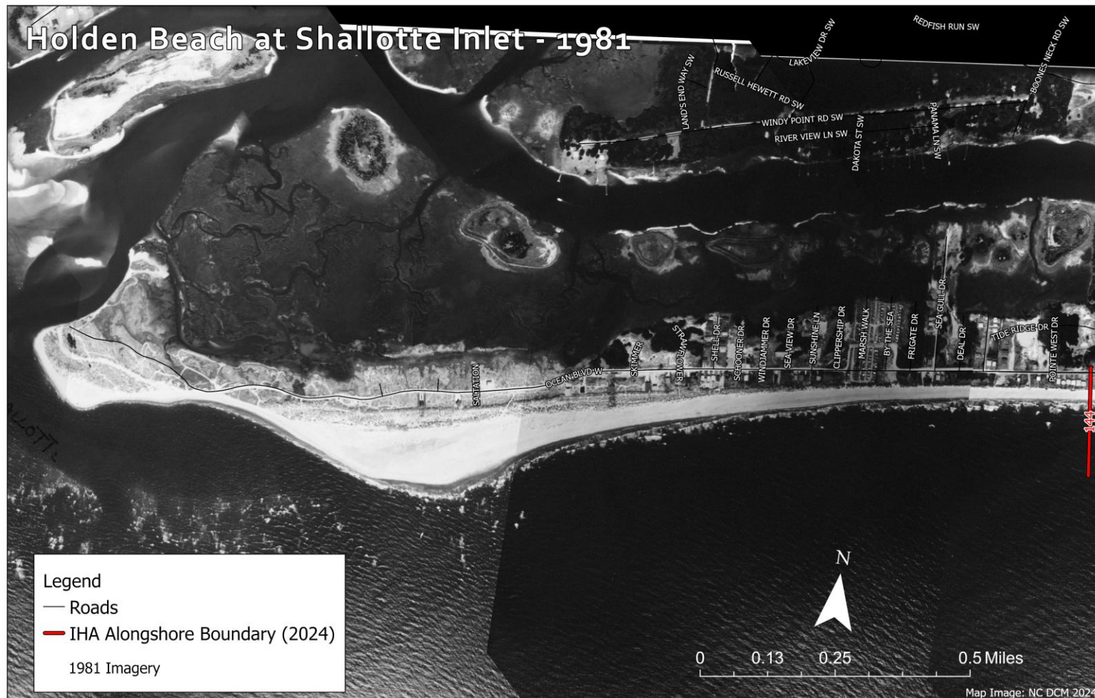
Figure D24. Shallotte Inlet at Holden Beach in 1981, shown relative to the 2024-2025 alongshore IHA boundary limit at transect 144 (marked by the red line on the right edge of the image). Note the bulbous area of accretion along the shoreline caused by the inlet's ebb channel orientation. This illustrates an accreting beach 21 years before the installation of the first major beach nourishment project.
