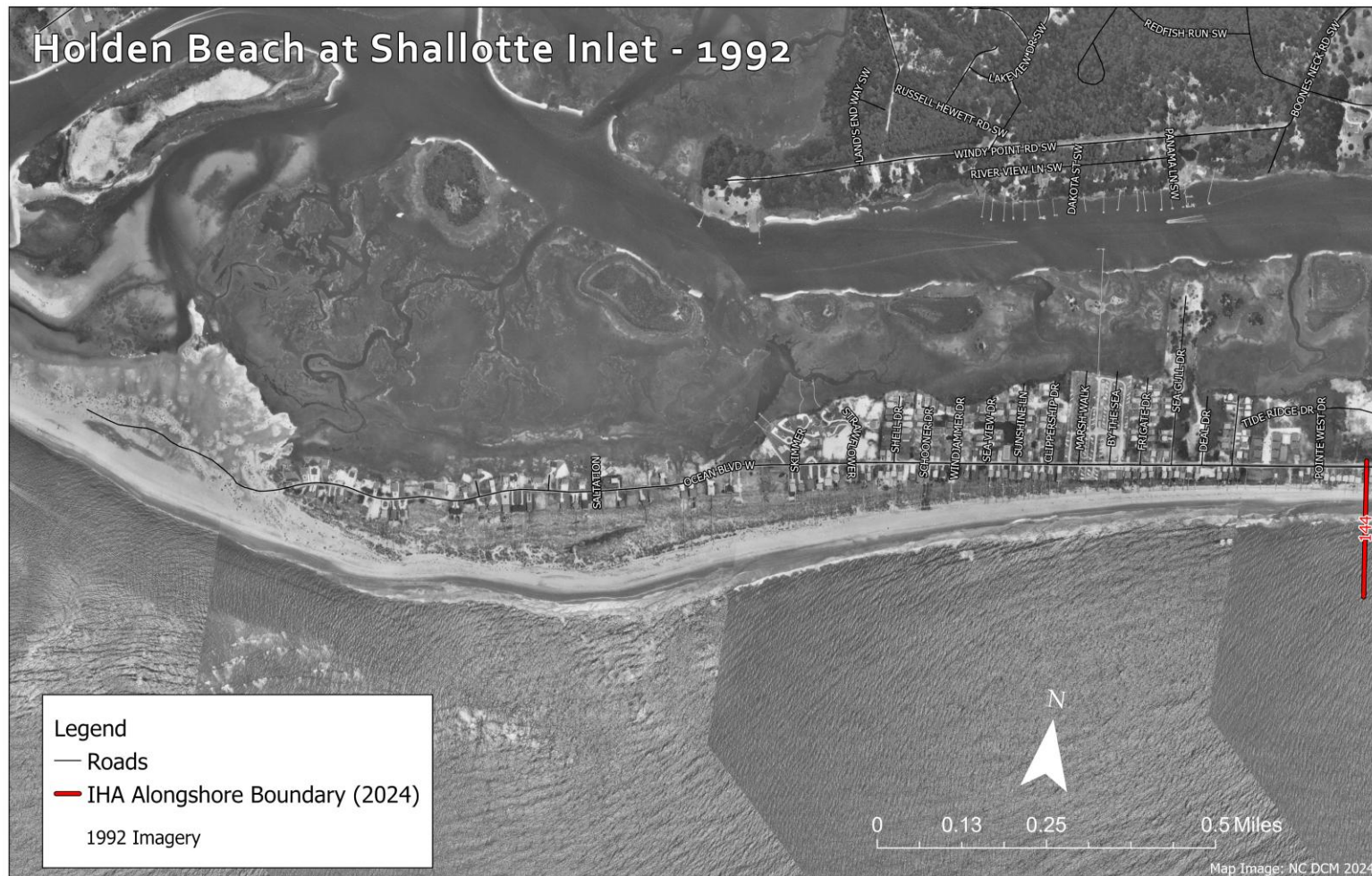
Figure D25. Shallotte Inlet at Holden Beach in 1992, shown relative to the 2024-2025 alongshore IHA boundary limit at transect 144 (marked by the red line on the right edge of the image), shows significant changes. Although the prominent accretion area is less noticeable due to short-term erosion and the growth of vegetation, the ebb channel along the shoreline remains visible. Additionally, gradual longshore accretion toward the alongshore IHA boundary is ongoing, indicating continued shoreline changes in this dynamic environment.
