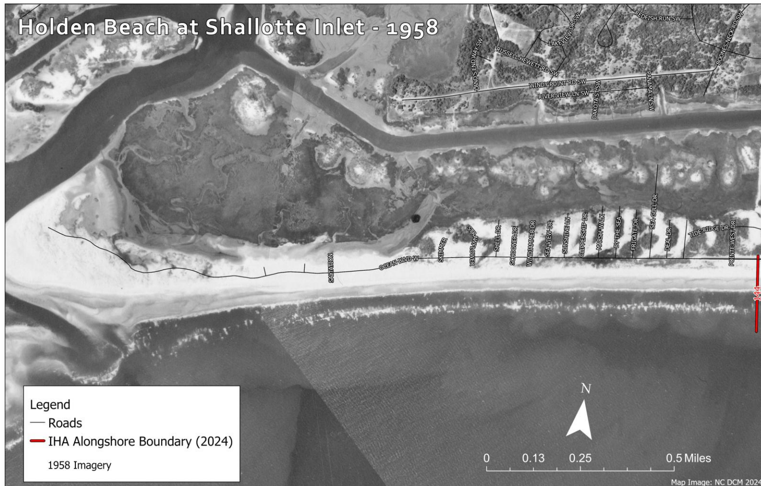
Figure D22. Shallotte Inlet at Holden Beach in 1958, shown relative to the 2024-2025 alongshore IHA boundary limit at transect 144 (marked by the red line on the right edge of the image). This image shows natural recovery over the course of four years following the breach and overwash associated with Hurricane Hazel. This photo is included for reference only as 1958 data were not use in the analysis.
