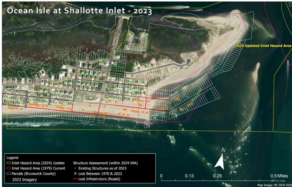
Figure 22. This map illustrates existing structures (green dots), and structures lost to erosion (houses indicated by red x-marks and roads indicated by red lines) relative to conditions in 2023. Based on an inventory for the period between 1970 and 2023, 58 structures and approximately 286 platted parcels and one mile of surfaced road within the 2024 IHA have been lost or relocated as a result of erosion. Currently, there are 185 structures within the 2024 IHA.
