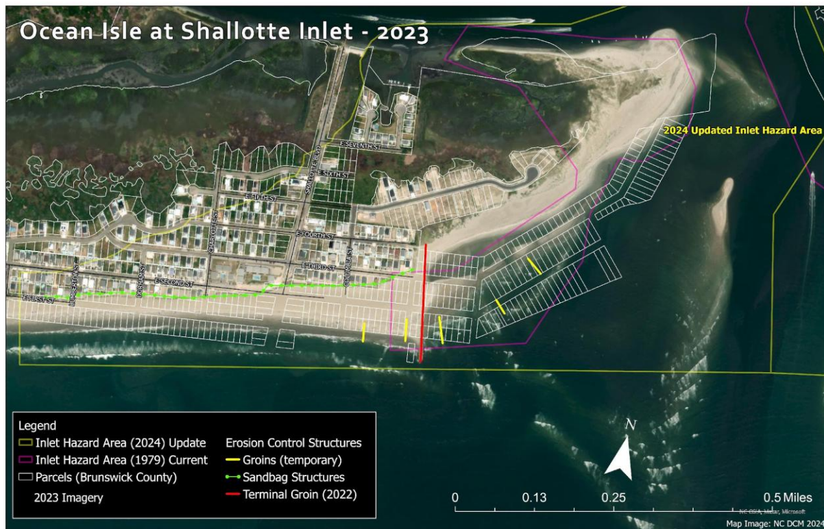
Figure 24. This map illustrates conditions in 2023 relative to the variety of erosion control structures applied in efforts to stabilize the shoreline. Small temporary groins (shore-perpendicular yellow lines) were installed before 1992 followed by sandbag structures (green dotted line) over the course of time, until construction of the terminal groin (red line) was completed in 2022.
