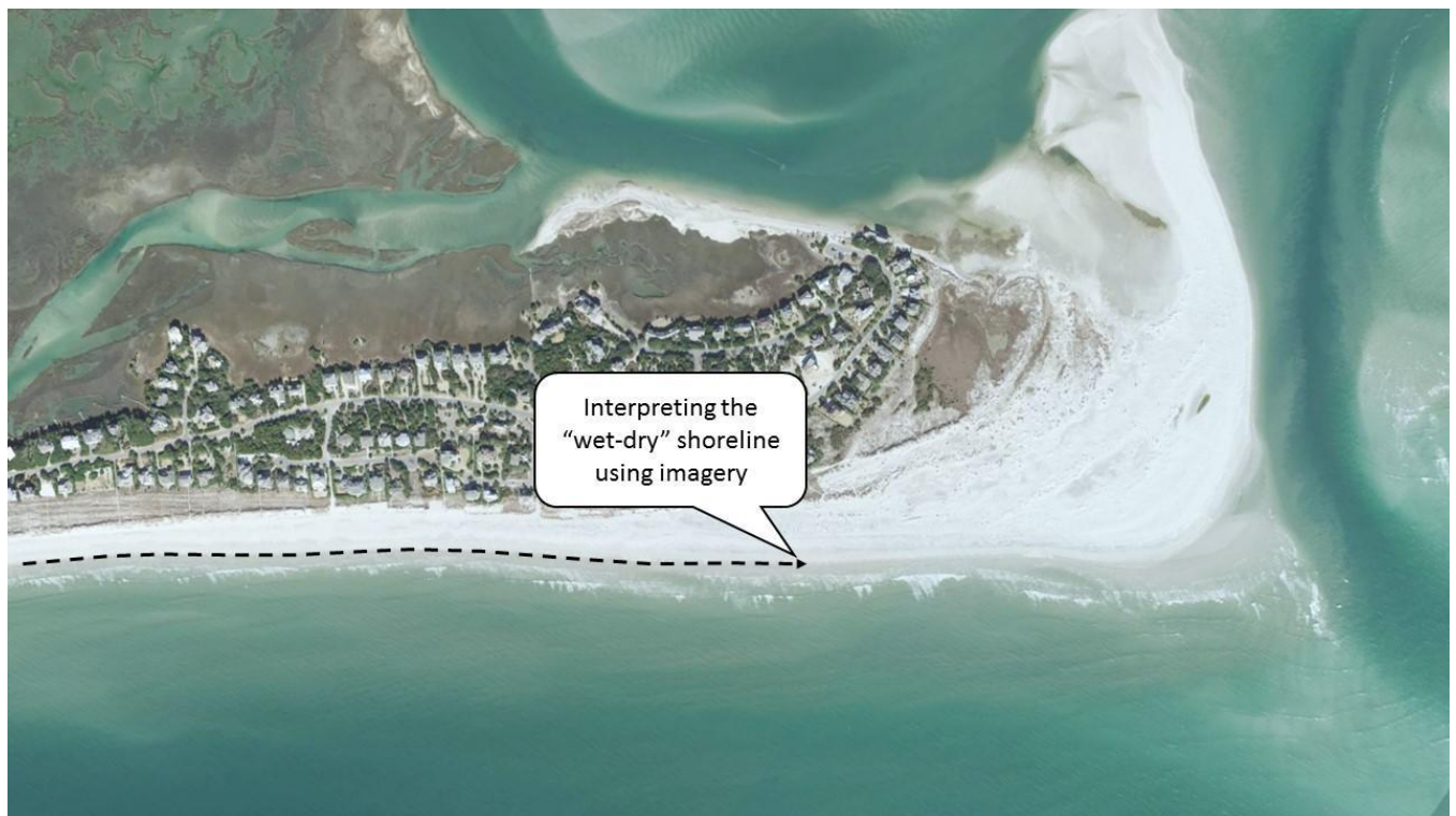
Figure 3. Interpretation of the "wet-dry" shoreline (black dashed line) using orthophotography.
