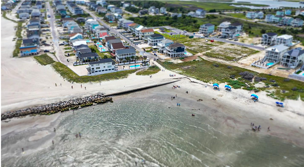
Figure 26. This image captures the inlet shoreline at the terminal groin as it appeared on June 25, 2024. Since 2023 (Figure 35), erosion on the inlet side of the groin has resulted in continued landward movement of the shoreline, exposing the groin's anchor, and approaching the vegetation in front of the new development. Photo source: NC DCM and DWR.
