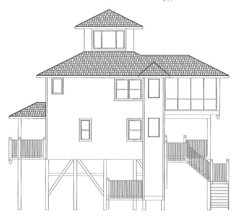
WEST ELEVATION EXISTING CONDITION WITH PROPOSED ELEVATOR
