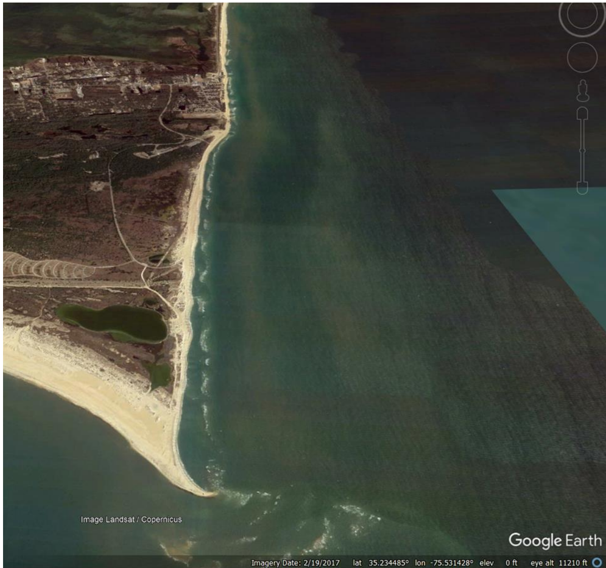
Figure 5. Oblique view of Buxton groins looking north from Cape Hatteras in 2017. When functional the groins have slowed the rate of erosion farther north with the tradeoff of creating a sand deficit farther south.
