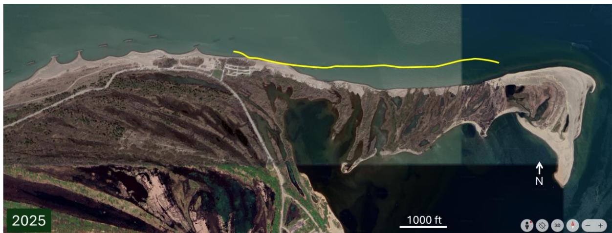
Figure 10. Presque Isle in 2006, 2016 and 2025 (top to bottom), showing continued, progressive erosion along the eastern end of the peninsula, downdrift of the field of breakwaters (Google Earth). The yellow curve in each image shows the shoreline position in 2006.
