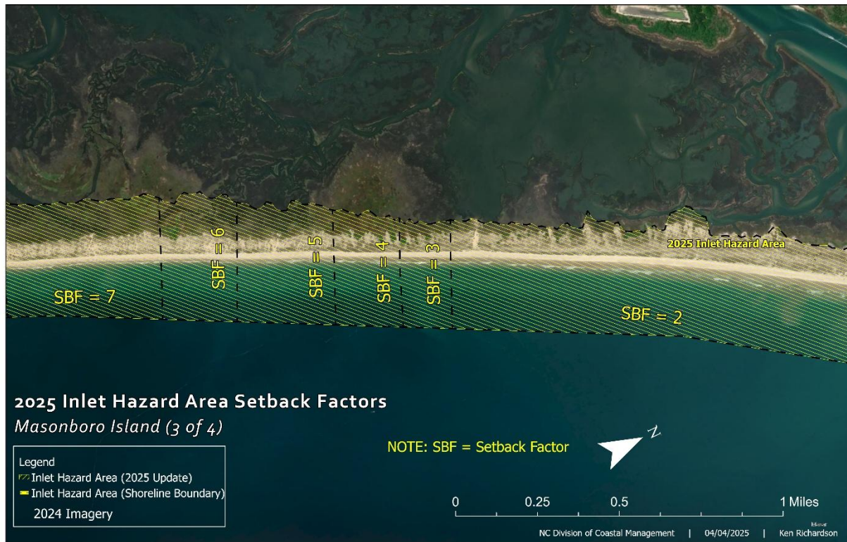
Figure 48. This map image illustrates 2025 inlet erosion setback factors in relation to the updated IHA boundary.
