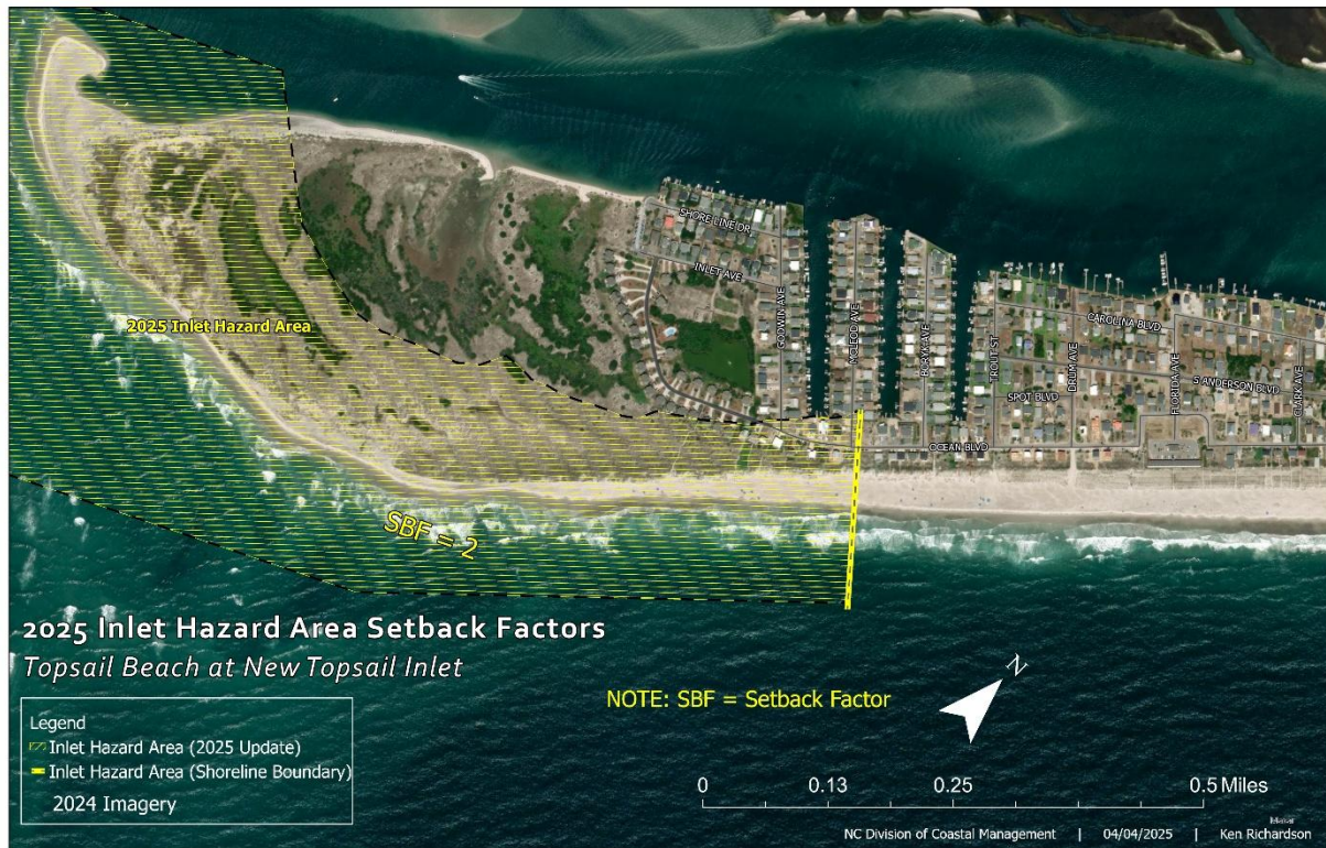
Figure 78. This map image illustrates 2025 inlet erosion setback factors in relation to the updated IHA boundary.
