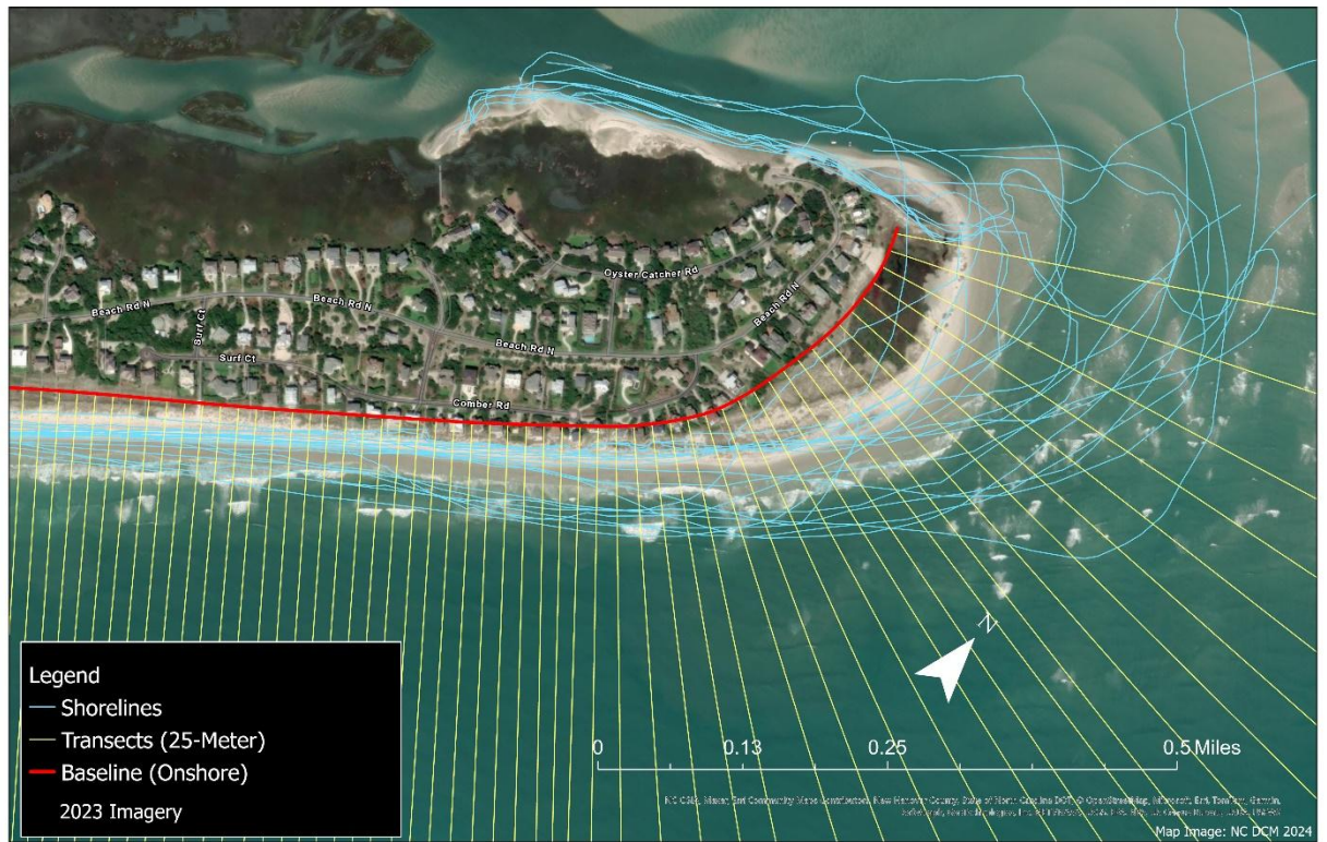
Figure 3. This map illustrates an example of casting 25-Meter transects (yellow line) from an onshore baseline (red line) that follows the general trend of shoreline positions.
