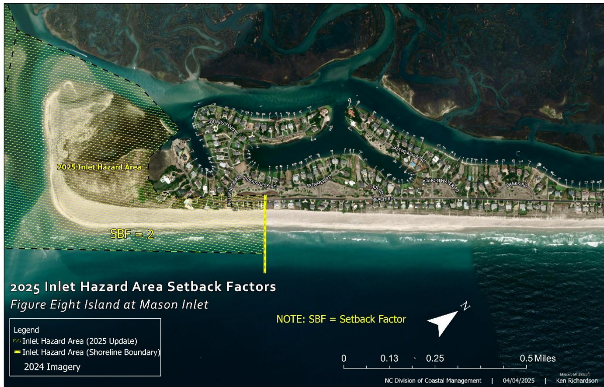
Figure 65. This map image illustrates 2025 inlet erosion setback factors in relation to the updated IHA boundary.
