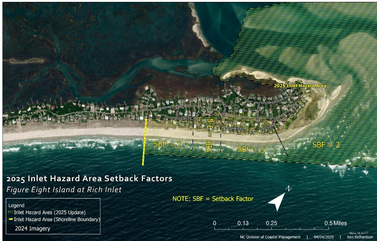
Figure 69. This map image illustrates 2025 inlet erosion setback factors in relation to the updated IHA boundary.
