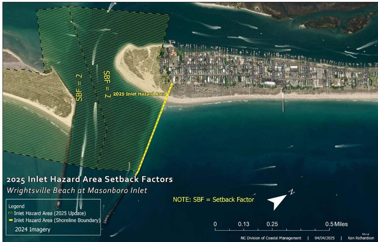
Figure 53. This map image illustrates 2025 inlet erosion setback factors in relation to the updated IHA boundary.
