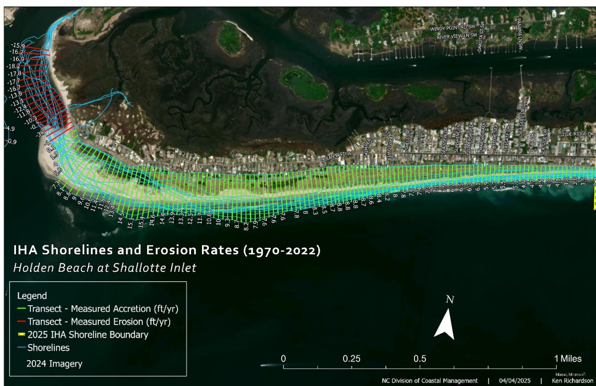
Figure 21. This map illustrates shorelines and erosion rates measured at each transect for the area approaching Shallotte Inlet from the 2025 updated IHA alongshore boundary (yellow transect).
