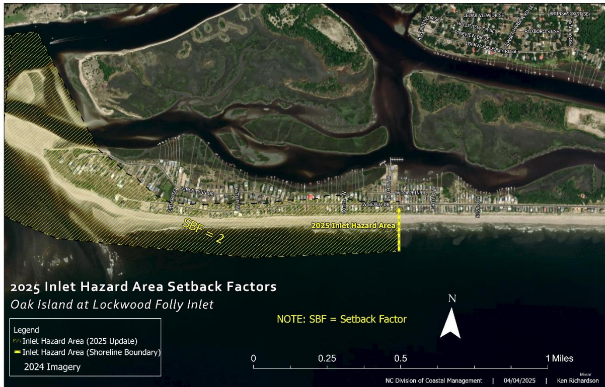
Figure 32. This map image illustrates 2025 inlet erosion setback factors in relation to the updated IHA boundary.
