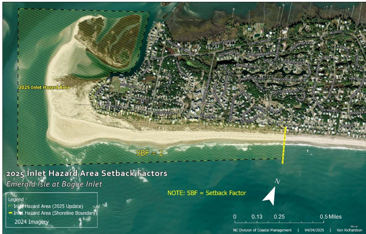
Figure 86. This map image illustrates 2025 inlet erosion setback factors in relation to the updated IHA boundary.
