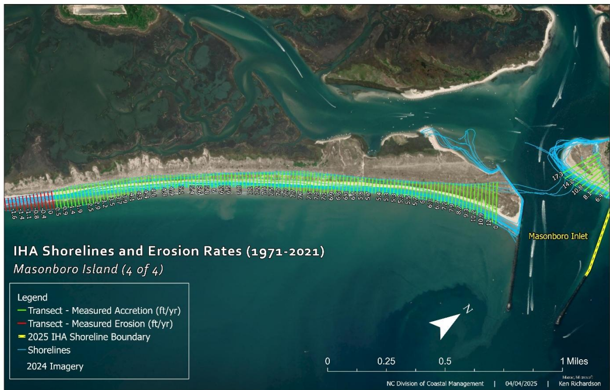
Figure 43. This map illustrates shorelines and erosion rates measured at each transect.
