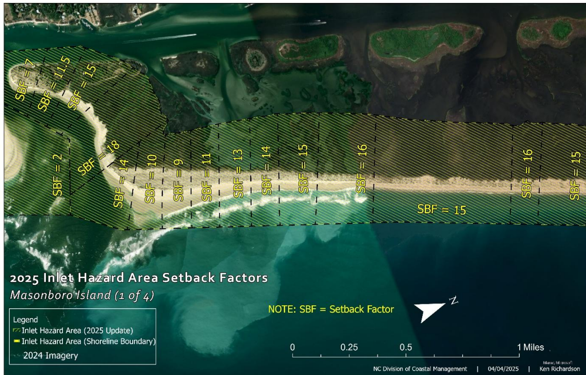
Figure 46. This map image illustrates 2025 inlet erosion setback factors in relation to the updated IHA boundary.
