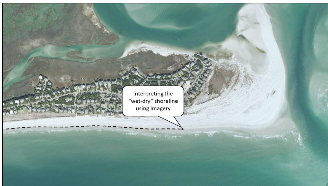
Figure 2. Interpretation of the "wet-dry" shoreline using orthophotography.
