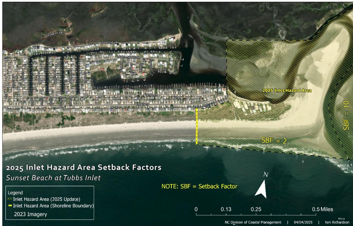
Figure 12. This map image illustrates 2025 inlet erosion rate setback factors in relation to the 2025 updated IHA boundary.
