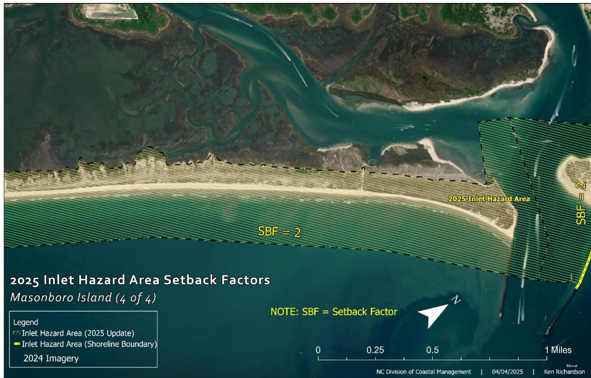
Figure 49. This map image illustrates 2025 inlet erosion setback factors in relation to the updated IHA boundary.
