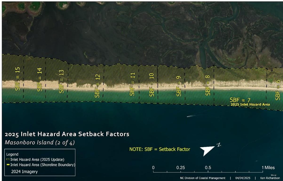
Figure 47. This map image illustrates 2025 inlet erosion setback factors in relation to the updated IHA boundary.
