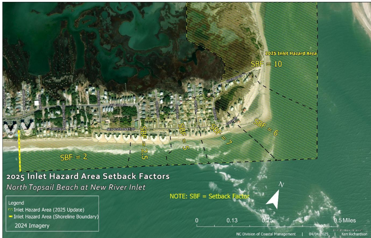
Figure 82. This map image illustrates 2025 inlet erosion setback factors in relation to the updated IHA boundary.
