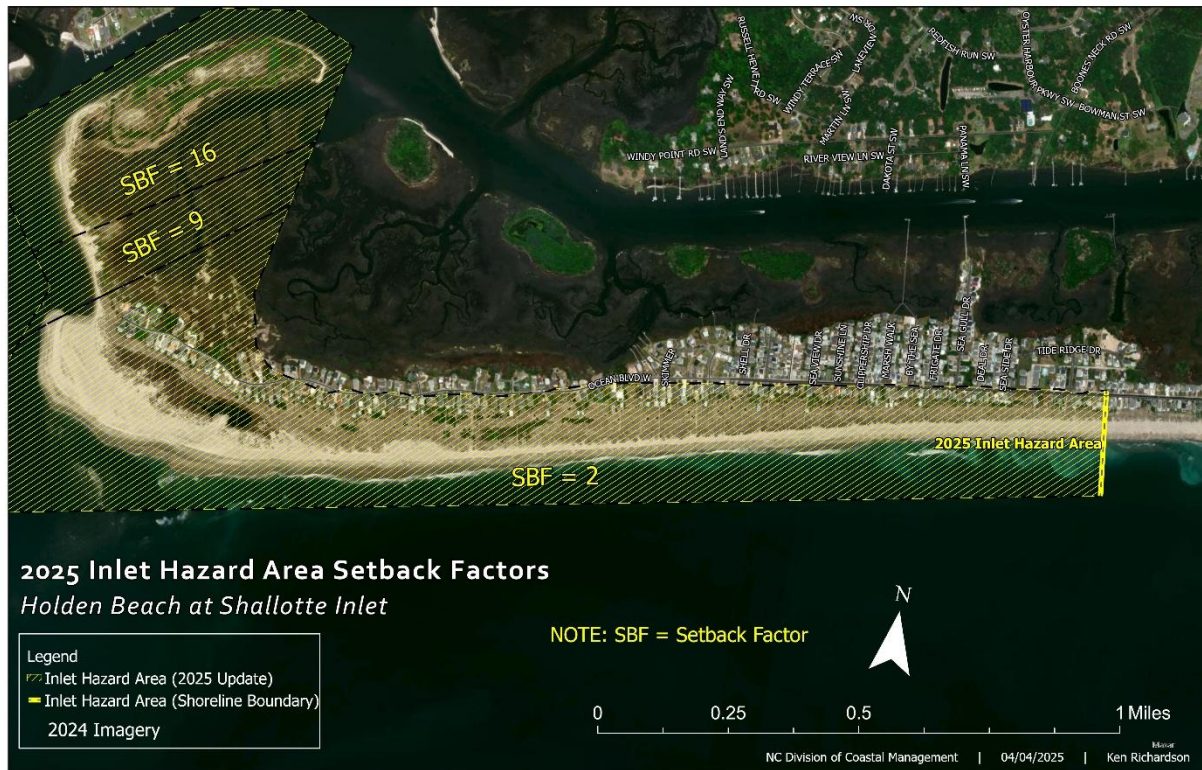
Figure 24. This map image illustrates 2025 inlet erosion setback factors in relation to the updated IHA boundary.
