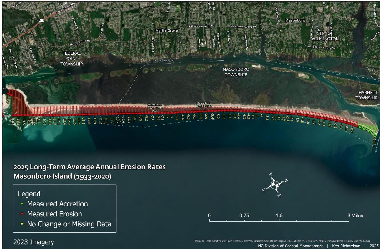
Figure 71. This map image illustrates the shoreline envelope at each transect, showing the area between the most oceanward and landward shorelines, labeled with erosion rates. Green lines indicate areas where accretion is measured, while red lines represent areas where erosion is measured using least squares regression.
