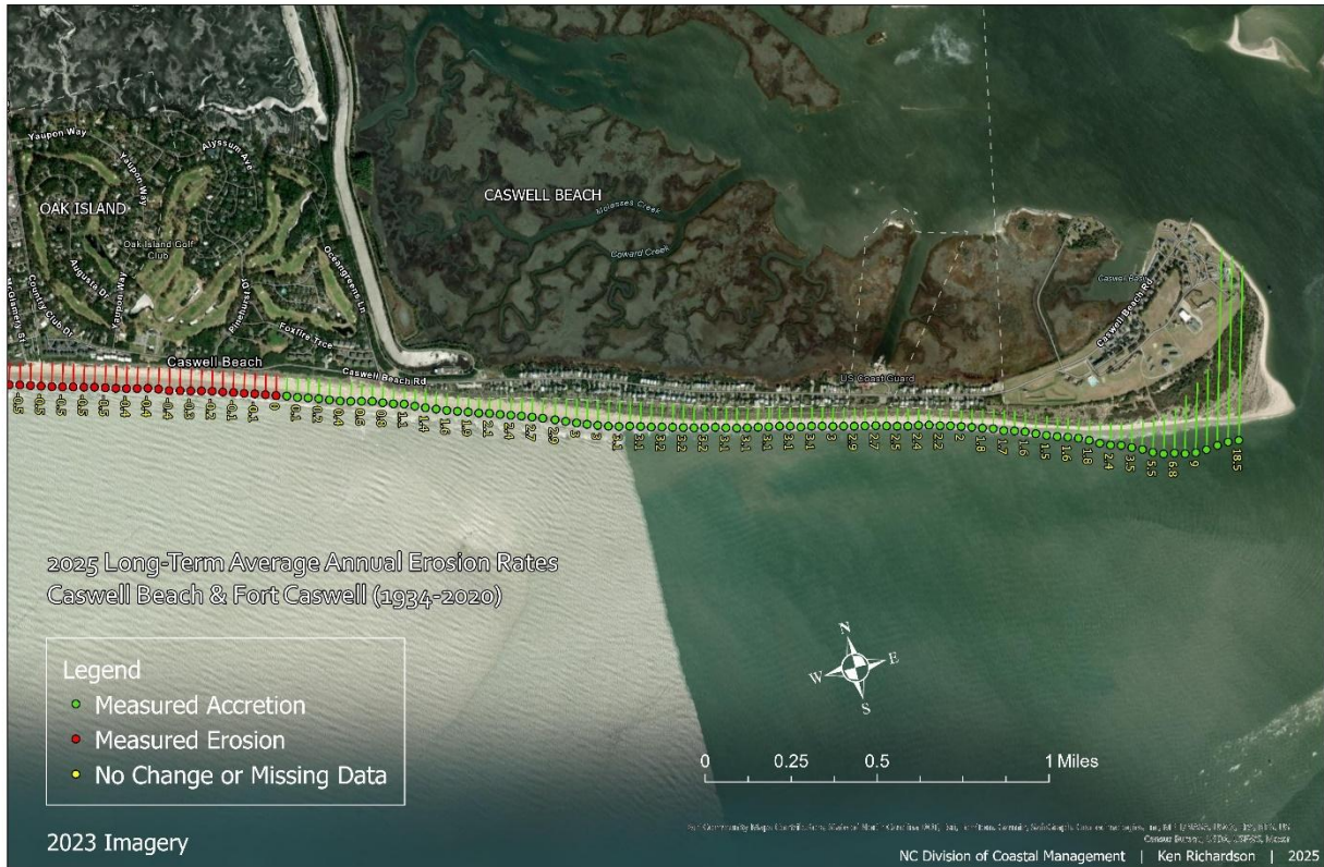
Figure 35. This map image illustrates the shoreline envelope at each transect, showing the area between the most oceanward and landward shorelines, labeled with erosion rates. Green lines indicate areas where accretion is measured, while red lines represent areas where erosion is measured using least squares regression.
