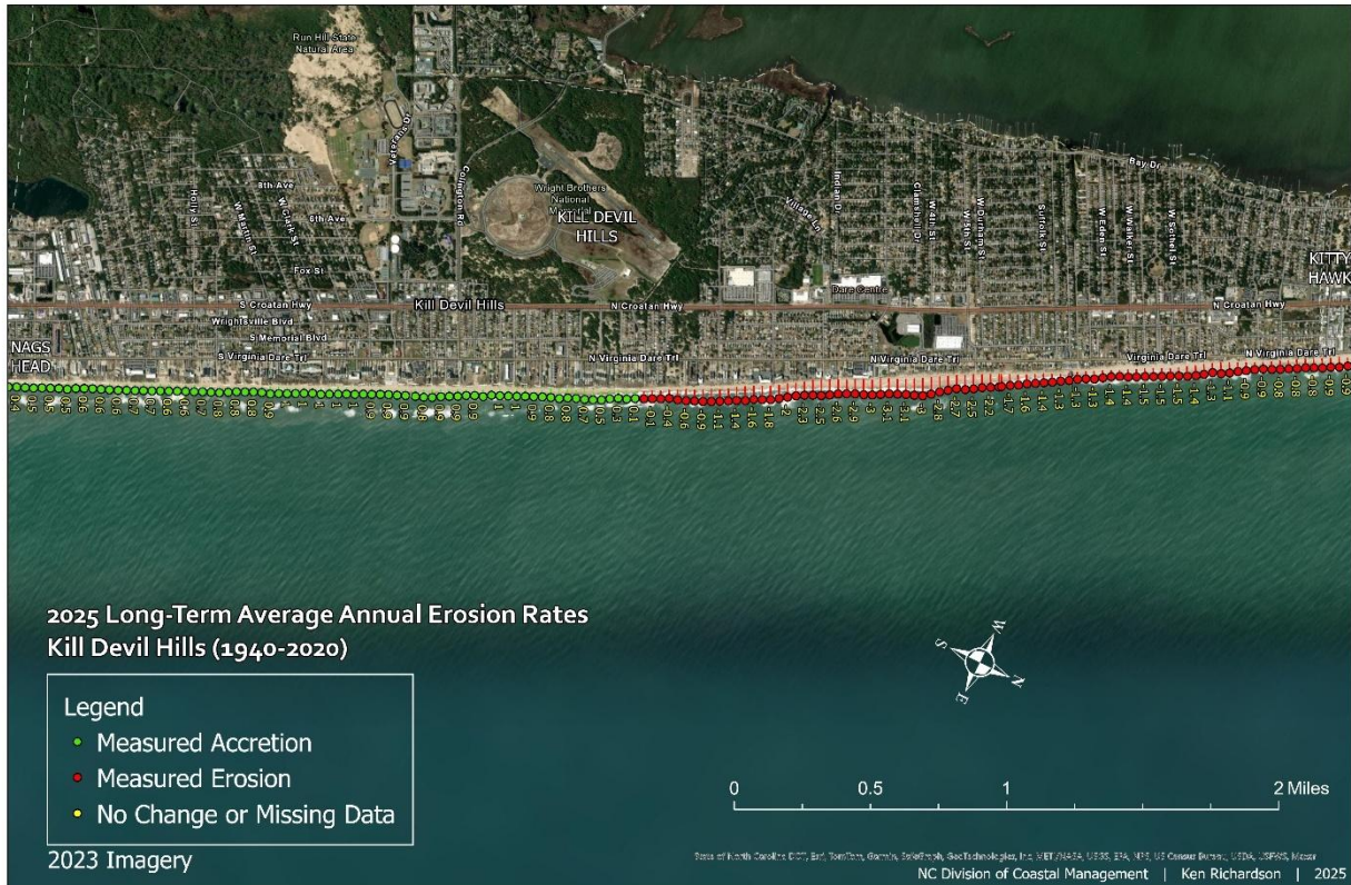
Figure 238. This map image illustrates the shoreline envelope at each transect, showing the area between the most oceanward and landward shorelines, labeled with erosion rates. Green lines indicate areas where accretion is measured, while red lines represent areas where erosion is measured using least squares regression.
