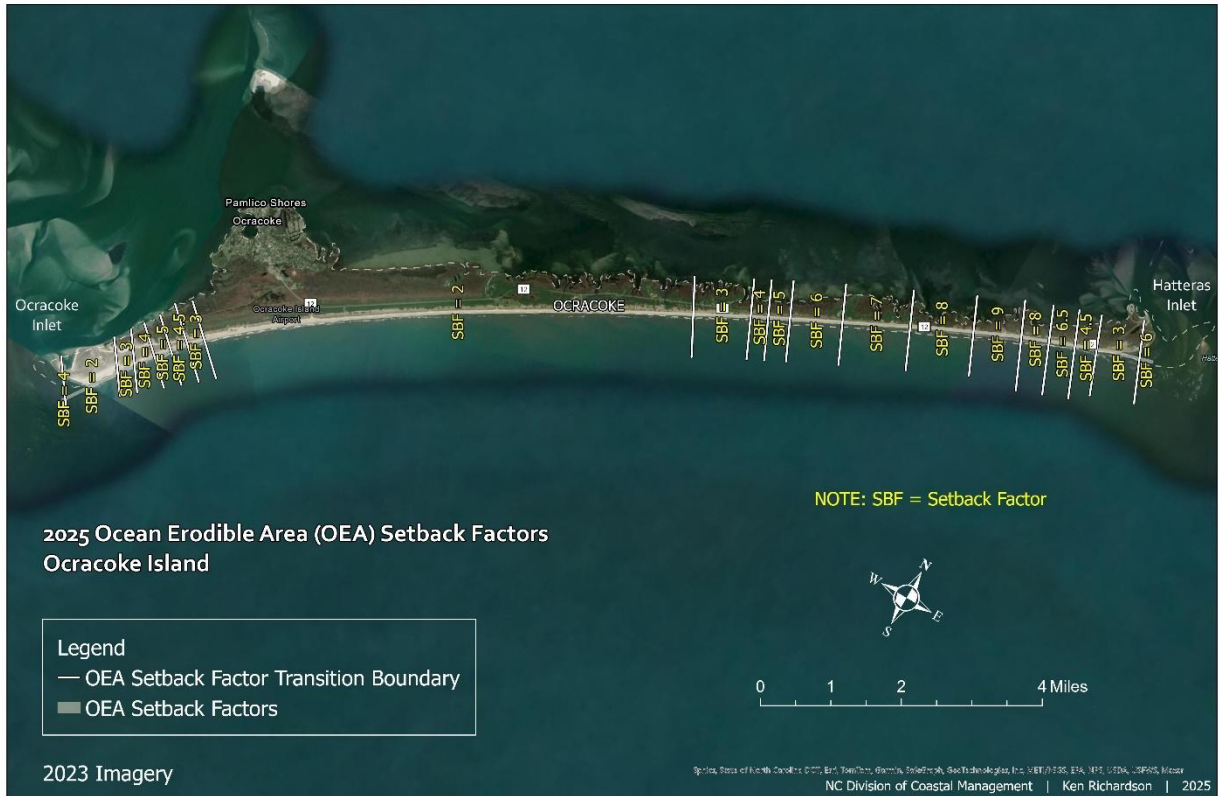
Figure 178. This map illustrates the erosion rate setback factors within the Ocean Erodible Area at Ocracoke Island.
