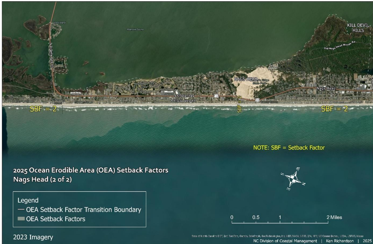
Figure 235. This map illustrates the erosion rate setback factors within the Ocean Erodible Area at Nags Head.
