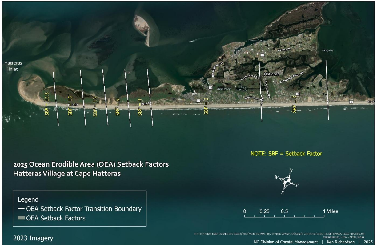
Figure 184. This map illustrates the erosion rate setback factors within the Ocean Erodible Area at Hatteras Village.
