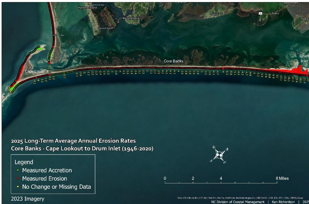
Figure 163. This map image illustrates the shoreline envelope at each transect, showing the area between the most oceanward and landward shorelines, labeled with erosion rates. Green lines indicate areas where accretion is measured, while red lines represent areas where erosion is measured using least squares regression.
