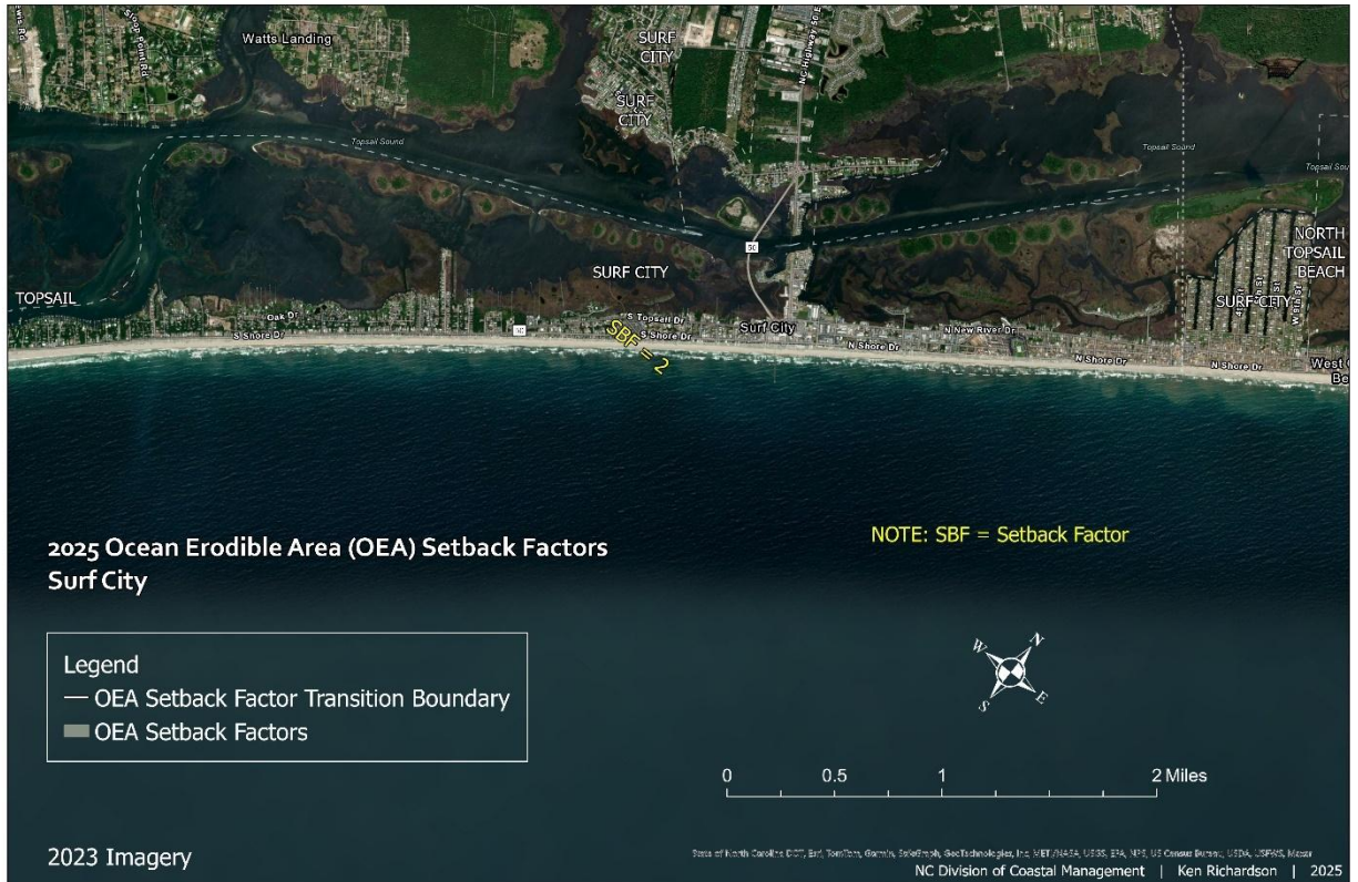
Figure 100. This map illustrates the erosion rate setback factors within the Ocean Erodible Area at Surf City. For setbacks within the proposed updated IHA boundary, refer to the report titled “NC Inlet Hazard Area (IHA) Erosion Rate & Setback Factors: 2025 Update.”
