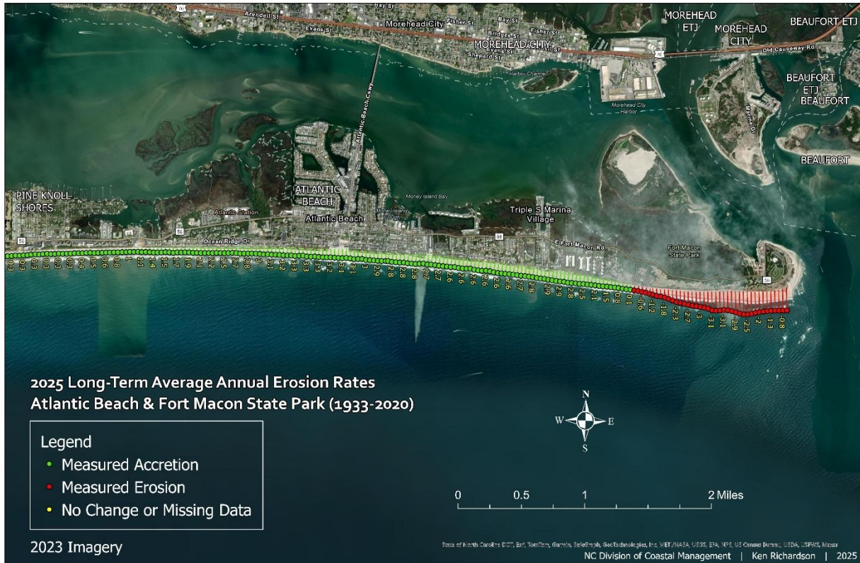
Figure 145. This map image illustrates the shoreline envelope at each transect, showing the area between the most oceanward and landward shorelines, labeled with erosion rates. Green lines indicate areas where accretion is measured, while red lines represent areas where erosion is measured using least squares regression.
