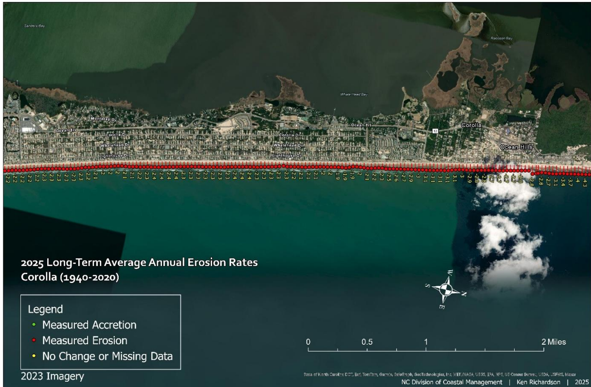
Figure 268. This map image illustrates the shoreline envelope at each transect, showing the area between the most oceanward and landward shorelines, labeled with erosion rates. Green lines indicate areas where accretion is measured, while red lines represent areas where erosion is measured using least squares regression.
