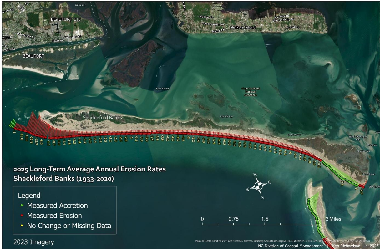
Figure 151. This map image illustrates the shoreline envelope at each transect, showing the area between the most oceanward and landward shorelines, labeled with erosion rates. Green lines indicate areas where accretion is measured, while red lines represent areas where erosion is measured using least squares regression.
