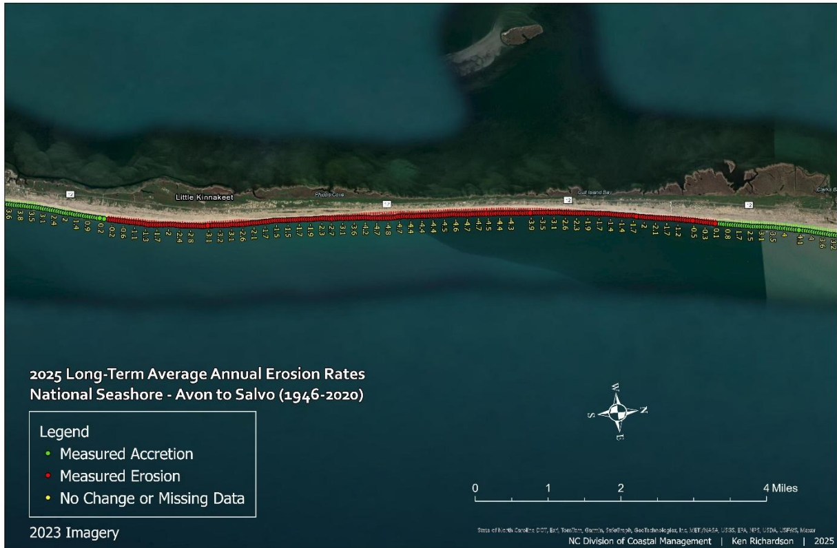
Figure 206. This map image illustrates the shoreline envelope at each transect, showing the area between the most oceanward and landward shorelines, labeled with erosion rates. Green lines indicate areas where accretion is measured, while red lines represent areas where erosion is measured using least squares regression.
