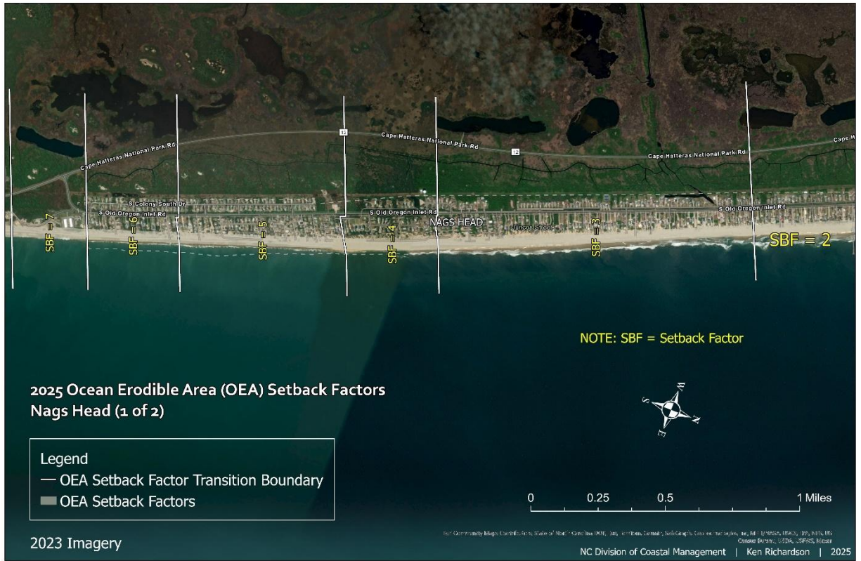
Figure 234. This map illustrates the erosion rate setback factors within the Ocean Erodible Area at Nags Head.
