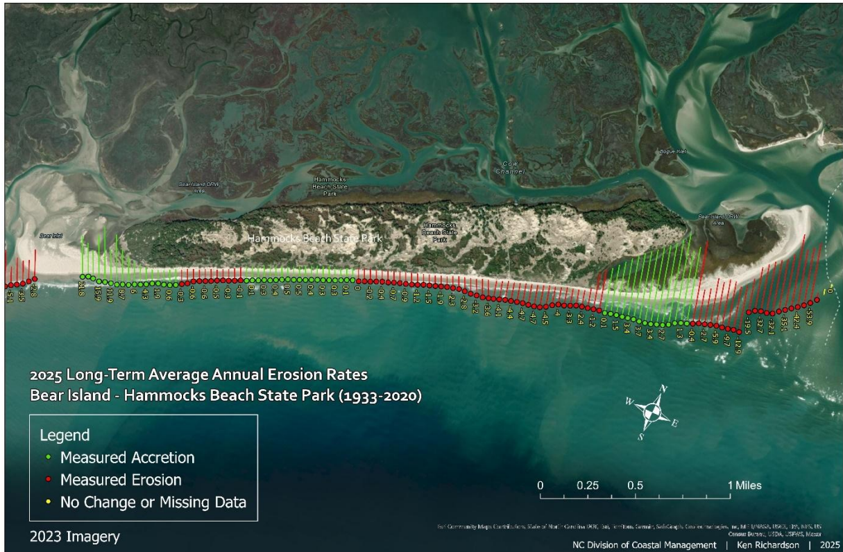
Figure 121. This map image illustrates the shoreline envelope at each transect, showing the area between the most oceanward and landward shorelines, labeled with erosion rates. Green lines indicate areas where accretion is measured, while red lines represent areas where erosion is measured using least squares regression.
