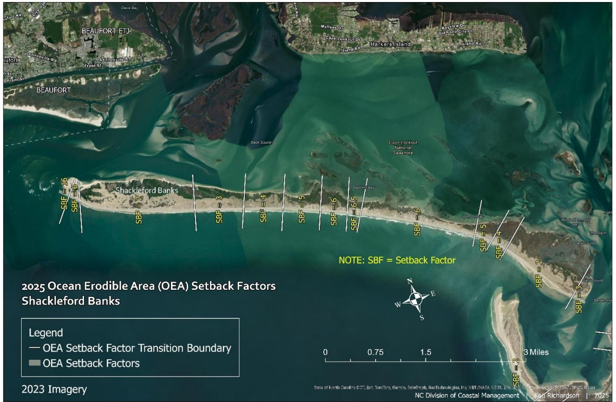
Figure 154. This map illustrates the erosion rate setback factors within the Ocean Erodible Area at Shackleford Banks.
