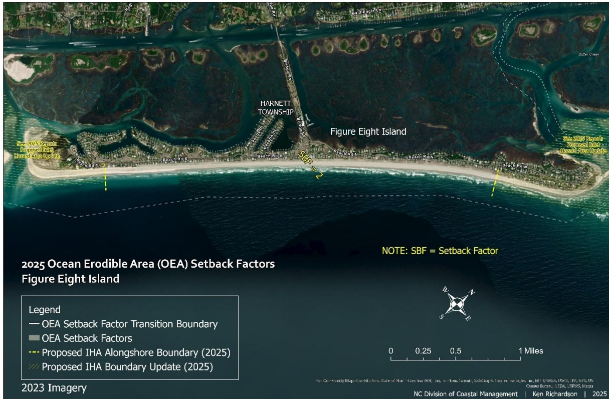
Figure 84. This map illustrates the erosion rate setback factors within the Ocean Erodible Area at Figure Eight Island. For setbacks within the proposed updated IHA boundary, refer to the report titled “NC Inlet Hazard Area (IHA) Erosion Rate & Setback Factors: 2025 Update.”
