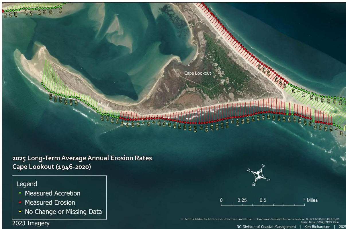
Figure 157. This map image illustrates the shoreline envelope at each transect, showing the area between the most oceanward and landward shorelines, labeled with erosion rates. Green lines indicate areas where accretion is measured, while red lines represent areas where erosion is measured using least squares regression.
