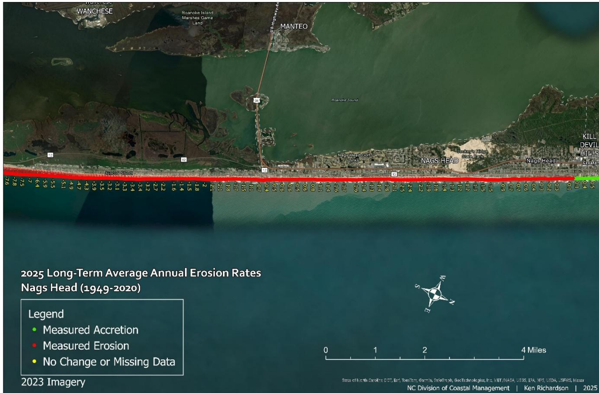
Figure 231. This map image illustrates the shoreline envelope at each transect, showing the area between the most oceanward and landward shorelines, labeled with erosion rates. Green lines indicate areas where accretion is measured, while red lines represent areas where erosion is measured using least squares regression.
