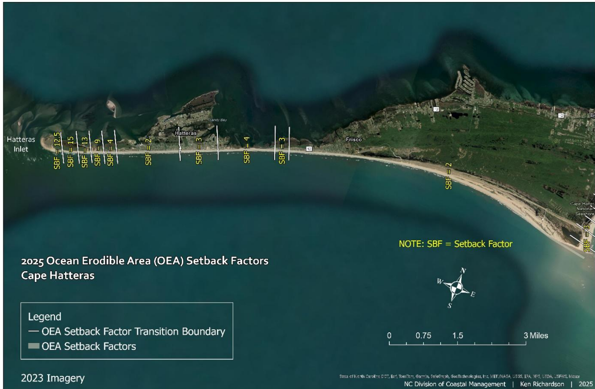
Figure 185. This map illustrates the erosion rate setback factors within the Ocean Erodible Area at Hatteras Inlet to Cape Hatteras.
