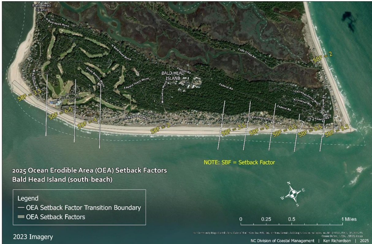
Figure 44. This map illustrates the erosion rate setback factors within the Ocean Erodible Area at Bald Head Island (south-beach).
