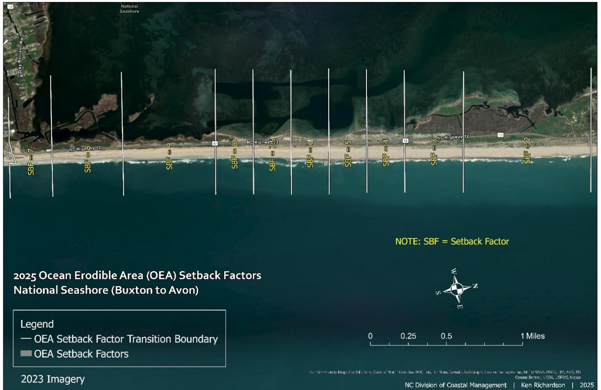
Figure 197. This map illustrates the erosion rate setback factors within the Ocean Erodible Area between Buxton and Avon.
