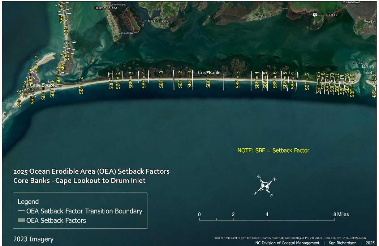
Figure 166. This map illustrates the erosion rate setback factors within the Ocean Erodible Area at Cape Lookout to Drum Inlet.
