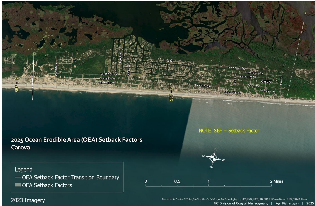
Figure 289. This map illustrates the erosion rate setback factors within the Ocean Erodible Area at Carova.
