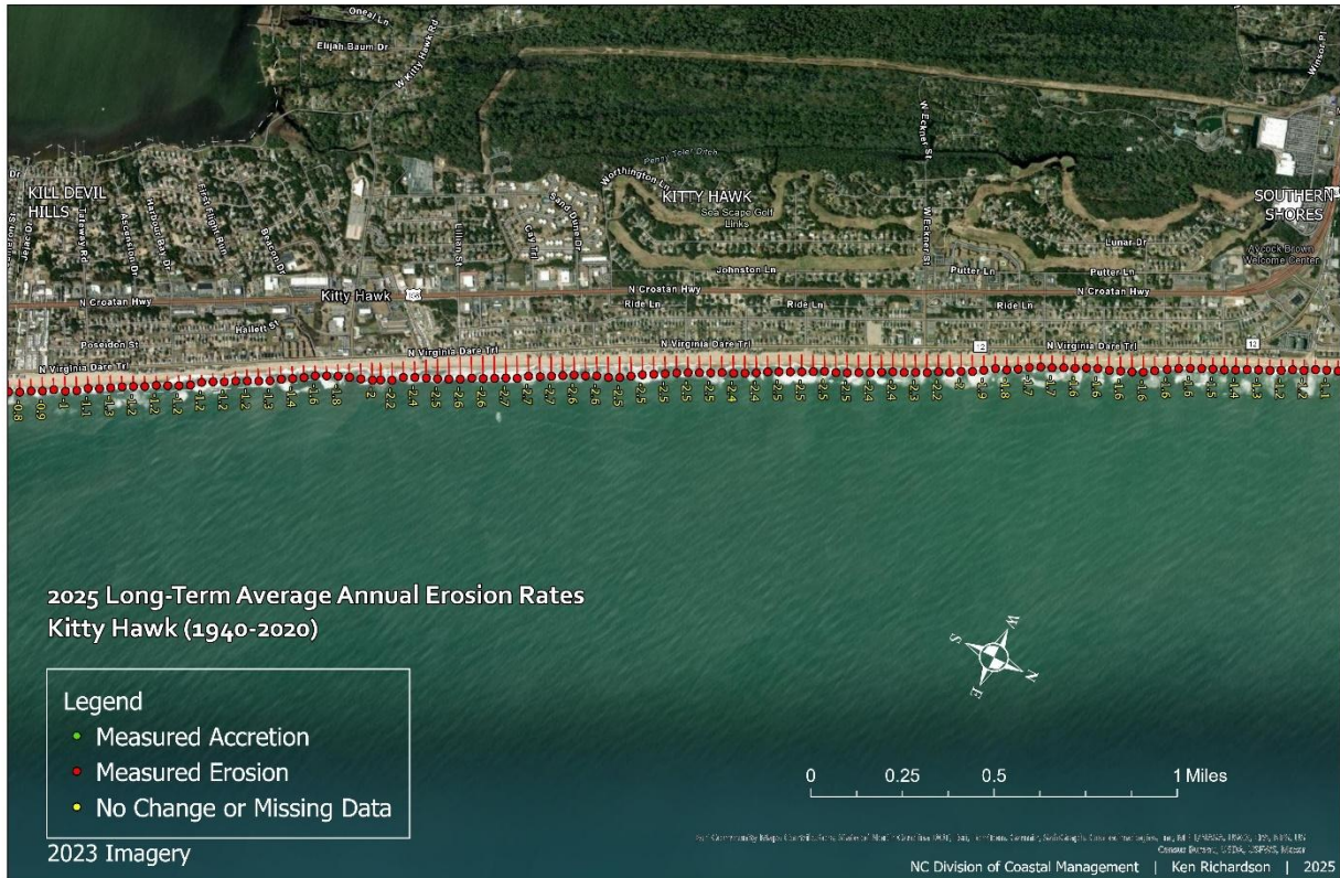
Figure 244. This map image illustrates the shoreline envelope at each transect, showing the area between the most oceanward and landward shorelines, labeled with erosion rates. Green lines indicate areas where accretion is measured, while red lines represent areas where erosion is measured using least squares regression.
