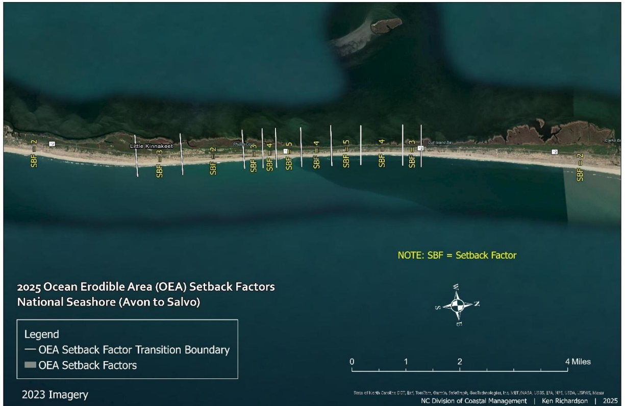
Figure 209. This map illustrates the erosion rate setback factors within the Ocean Erodible Area between Avon and Salvo.
