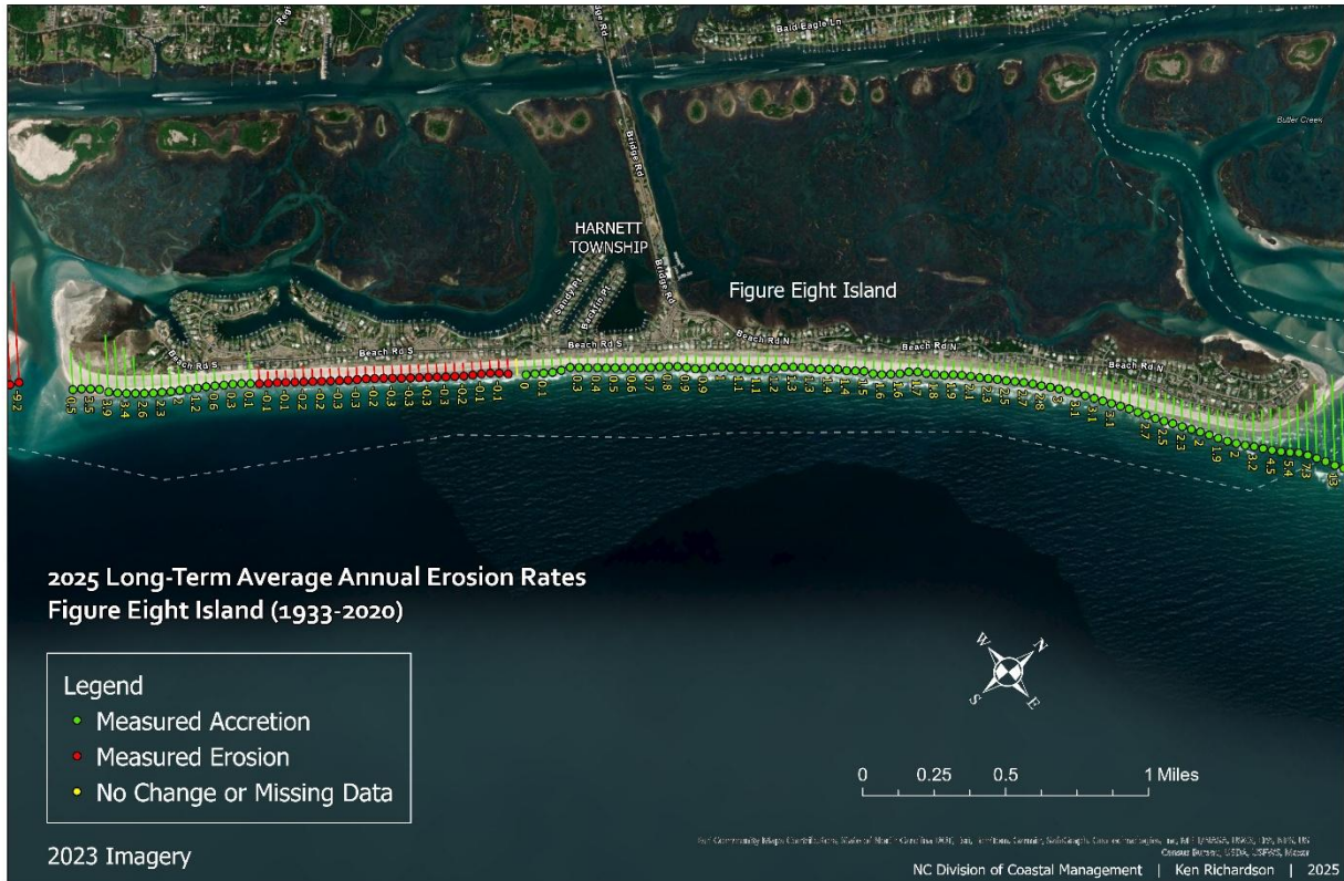
Figure 81. This map image illustrates the shoreline envelope at each transect, showing the area between the most oceanward and landward shorelines, labeled with erosion rates. Green lines indicate areas where accretion is measured, while red lines represent areas where erosion is measured using least squares regression.
