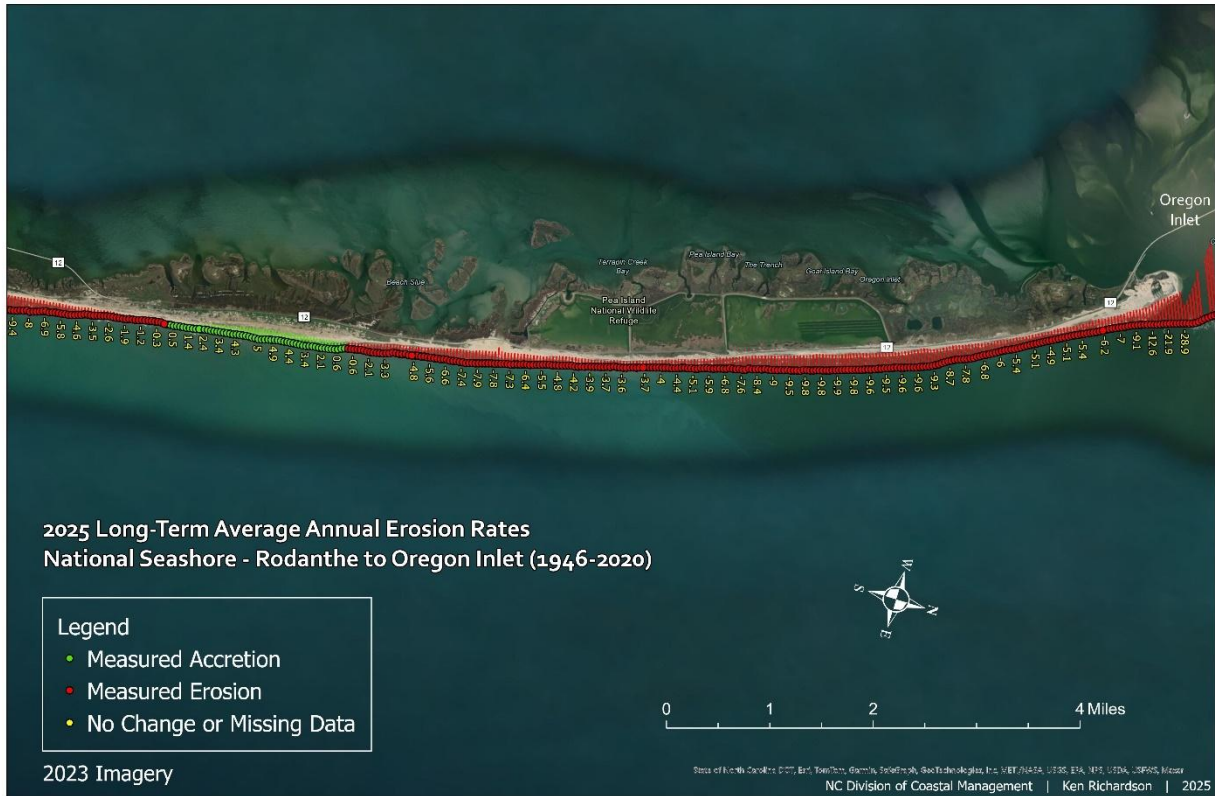
Figure 219. This map image illustrates the shoreline envelope at each transect, showing the area between the most oceanward and landward shorelines, labeled with erosion rates. Green lines indicate areas where accretion is measured, while red lines represent areas where erosion is measured using least squares regression.
