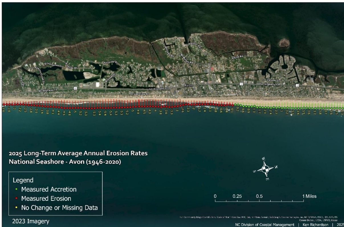
Figure 200. This map image illustrates the shoreline envelope at each transect, showing the area between the most oceanward and landward shorelines, labeled with erosion rates. Green lines indicate areas where accretion is measured, while red lines represent areas where erosion is measured using least squares regression.
