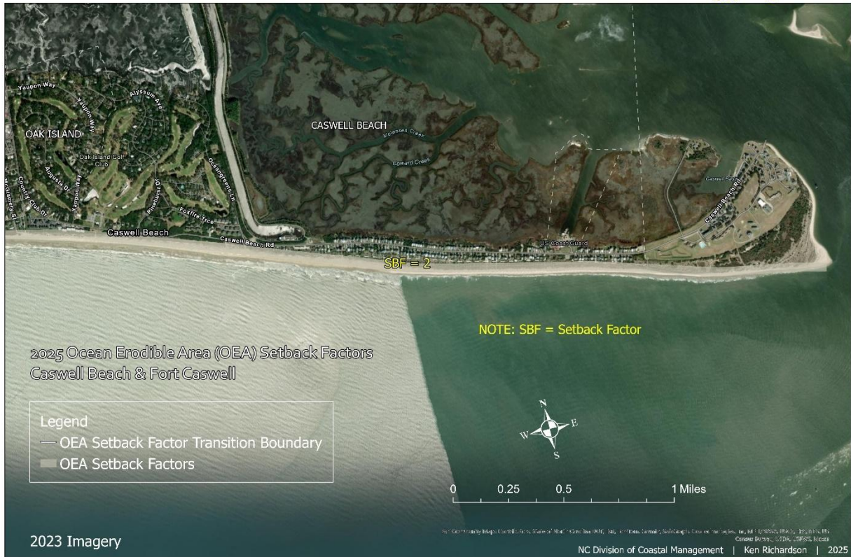
Figure 38. This map illustrates the erosion rate setback factors within the Ocean Erodible Area at Caswell Beach and Fort Caswell.
