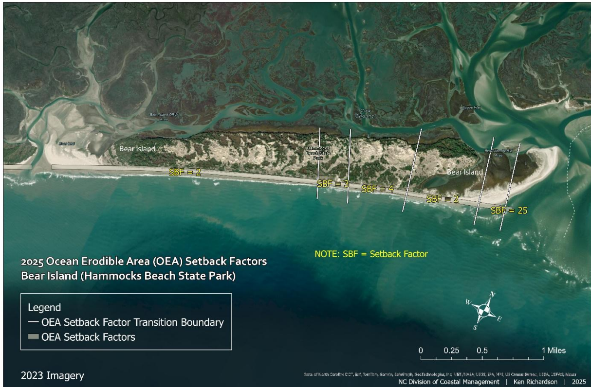
Figure 124. This map illustrates the erosion rate setback factors within the Ocean Erodible Area at Bear Island (Hammocks Beach State Park). For setbacks within the proposed updated IHA boundary, refer to the report titled “NC Inlet Hazard Area (IHA) Erosion Rate & Setback Factors: 2025 Update.”
