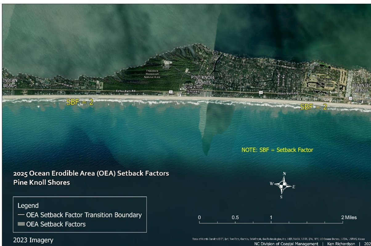
Figure 142. This map illustrates the erosion rate setback factors within the Ocean Erodible Area at Pine Knoll Shores.
