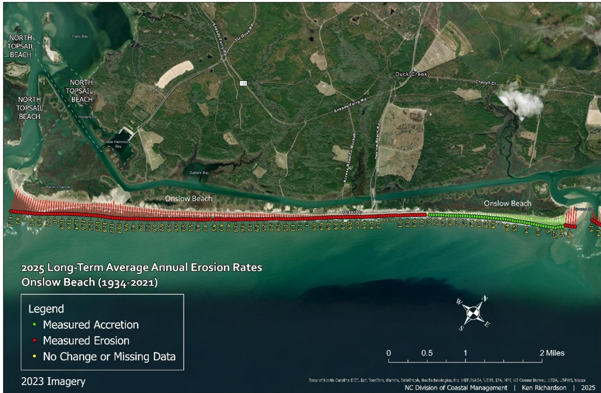
Figure 109. This map image illustrates the shoreline envelope at each transect, showing the area between the most oceanward and landward shorelines, labeled with erosion rates. Green lines indicate areas where accretion is measured, while red lines represent areas where erosion is measured using least squares regression.
