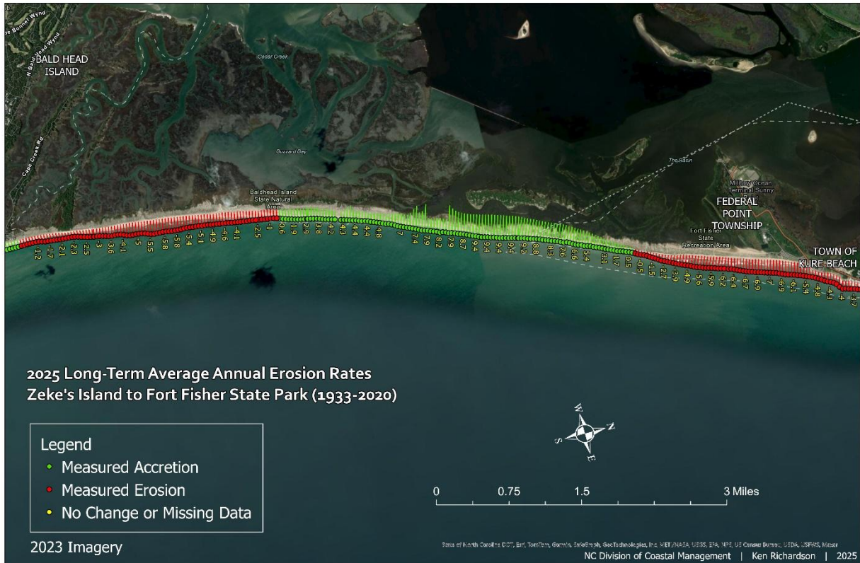
Figure 53. This map image illustrates the shoreline envelope at each transect, showing the area between the most oceanward and landward shorelines, labeled with erosion rates. Green lines indicate areas where accretion is measured, while red lines represent areas where erosion is measured using least squares regression.
