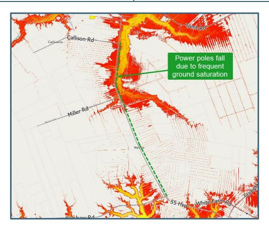
Figure 16: Proposed undergrounding of powerlines along Callison Road
