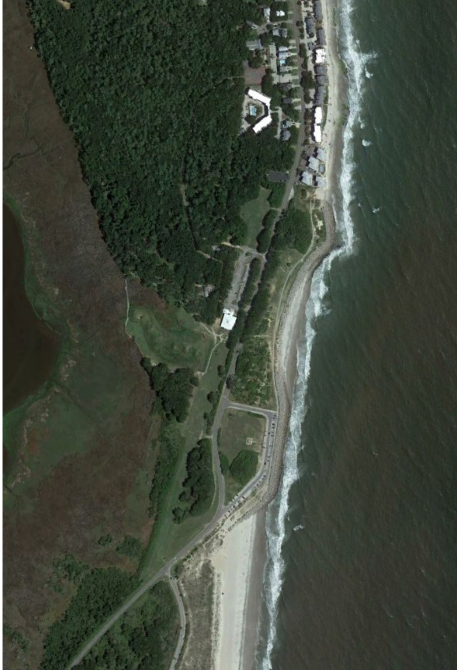
Figure 3. Fort Fisher, fronted by a revetment that now extends seaward past the position of the beach to the south, without a beach in front. A pocket beach in the cove between the revetment and the rocky headland to the north formed after a Kure Beach nourishment project.
