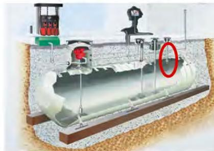
A ball float allows vapor and air to escape as the tank is filled. When the fuel reaches the ball float and lifts it up, it blocks the airflow out of the pipe above. This changes the flow rate and the driver can notice the difference and know the tank is near full.
