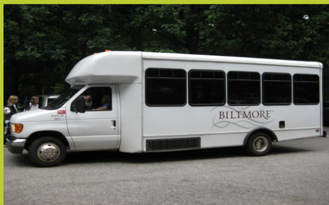
The 6.8L, V-10 Starcraft Allstar 25 shuttle bus (shown above) now runs primarily on propane and can fill up from the on-site Alliance AutoGas tank (shown below) near the security building.
