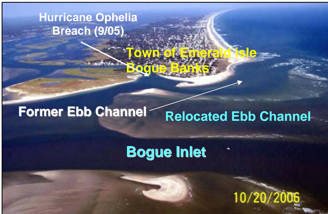
Figure IX-35. Bogue Inlet Ebb Channel Realignment (Cleary, 2008)
