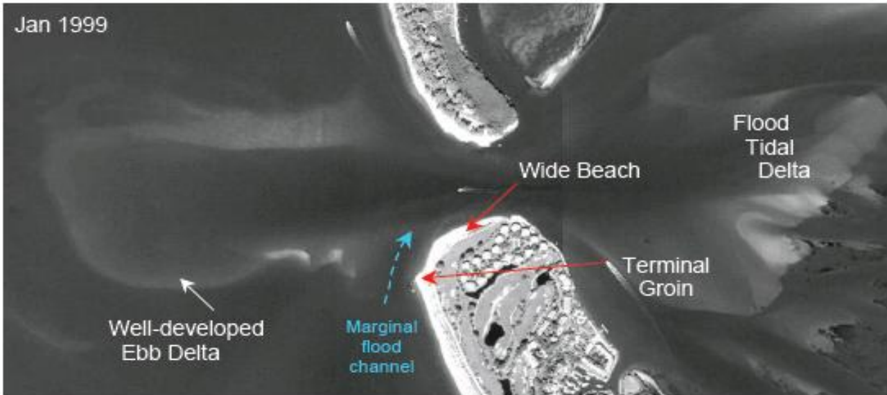
Figure II-55. View of the Ebb-tidal Delta That Has Been Used as a Source of Sand for Nourishing the Beach Along Captiva Island (from Google Earth)
