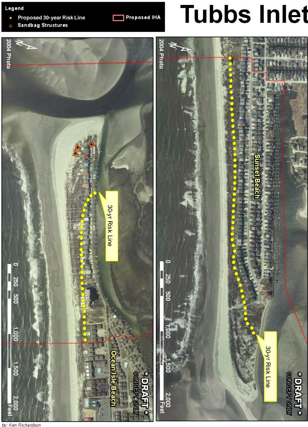
Figure V-12. 30-yr Risk Line and Sandbags at Tubbs Inlet
