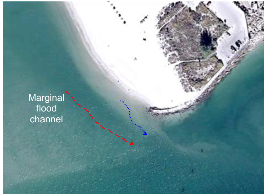
Figure II-71. Vertical Aerial Photograph of the Terminal Groin at the North Side of John's Pass
