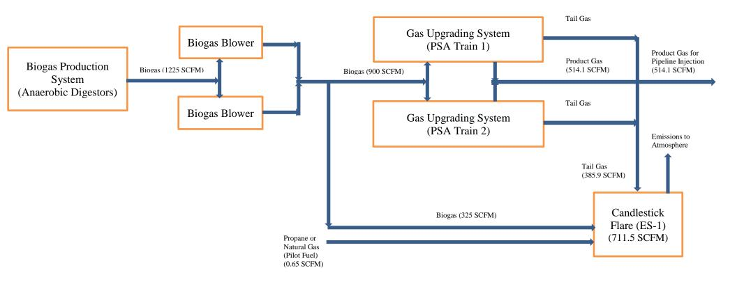
Process Flow Diagram Operating Scenario 2: Bypass Operation (240 hours)
