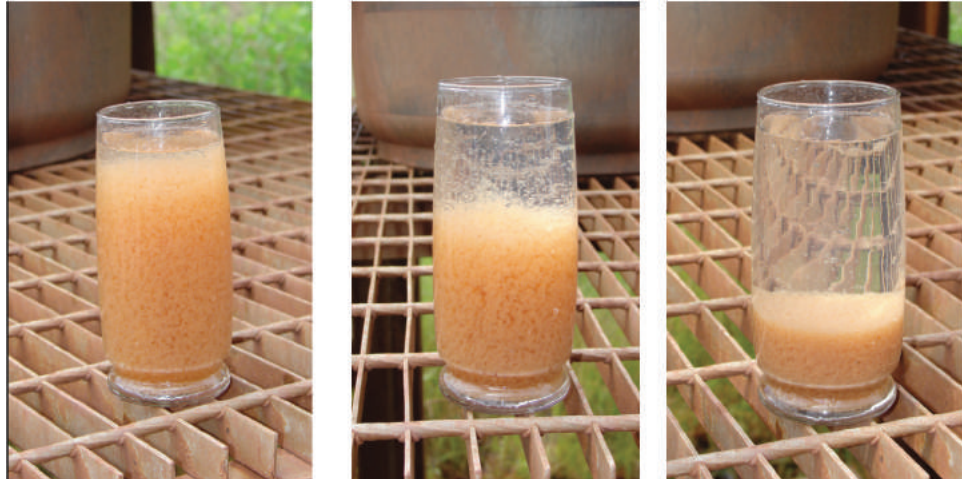
Figure 6.86a Flocculation of sediment with PAM.
