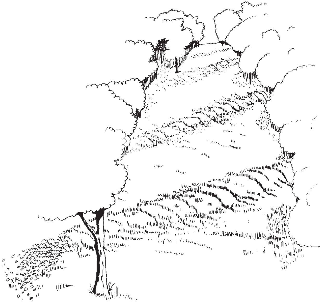
Figure 6.23a Water bars to protect utility right-of-way.
