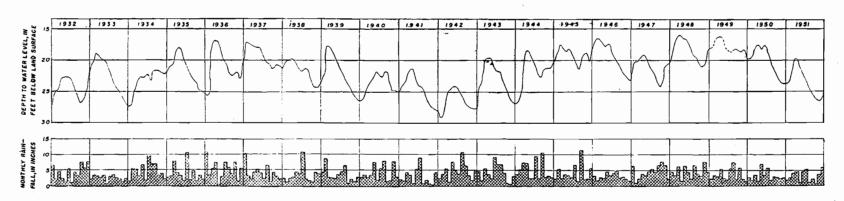
FIGURE 5.—Chart showing fluctuation of the water level in a dug well at Mocksville, Davie County. The well, owned by L. S. Kurfees, is 32 feet deep.
