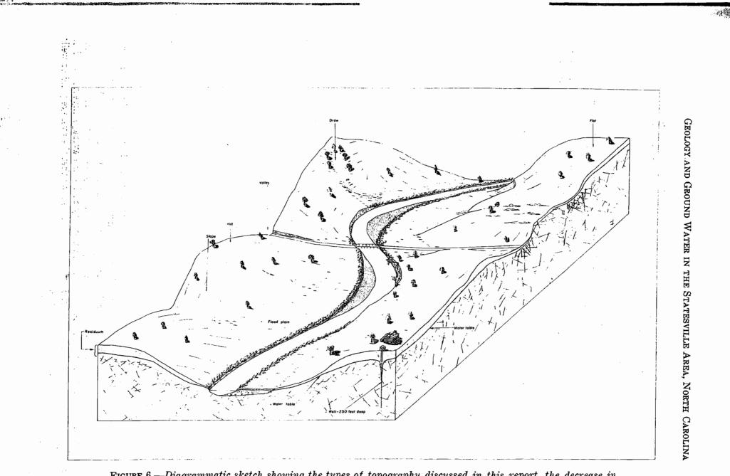
FIGURE 6.—Diagrammatic sketch showing the types of topography discussed in this report, the decrease in joints with increasing depth in the bedrock, and some of the interrelations of the residuum, the water table, and the topography.
