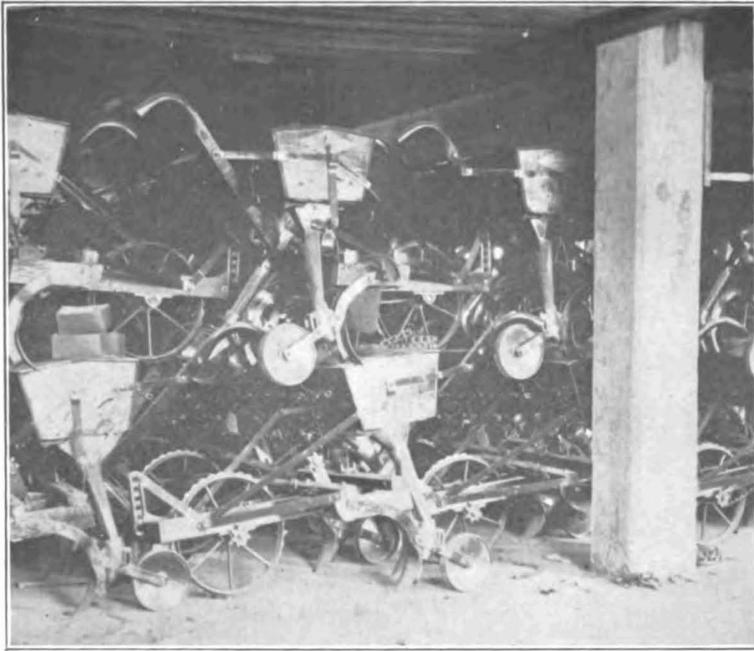
A. One-horse, three-row grain drills as manufactured in an agricultural implement factory of North Carolina. Oak is used for handles and beams, while North Carolina pine is employed for seed boxes.
