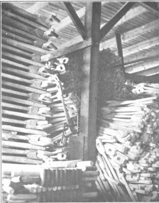
B. Finished and partly finished "D" shovel handles in a North Carolina handle plant.
