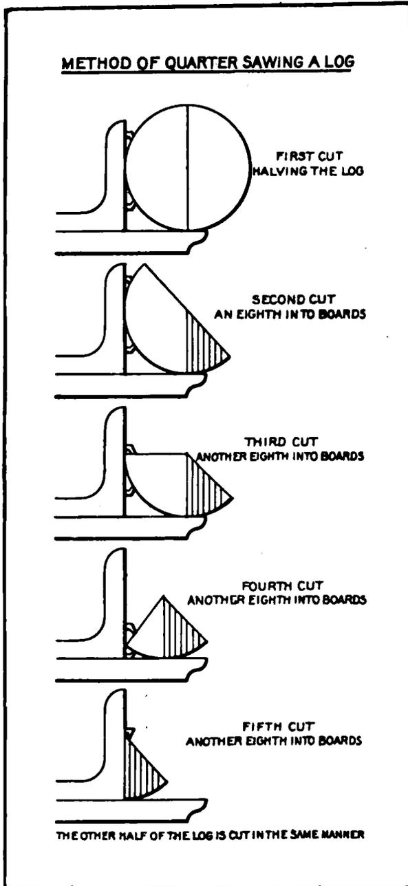
PLATE No. 26—Method of quarter-sawing a log.
