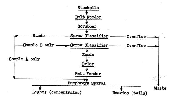
As noted in the flowsheet, the sands from Sample A were washed in only one screw classifier before being sent to the spiral. When running Sample B, the flowsheet was cut into two parts. The sand was scrubbed and washed in two classifiers and then dried before feeding to the spiral with a belt feeder. This was necessary because the desired feed rate to the spiral was three times the maximum feed rate to the scrubbers.
