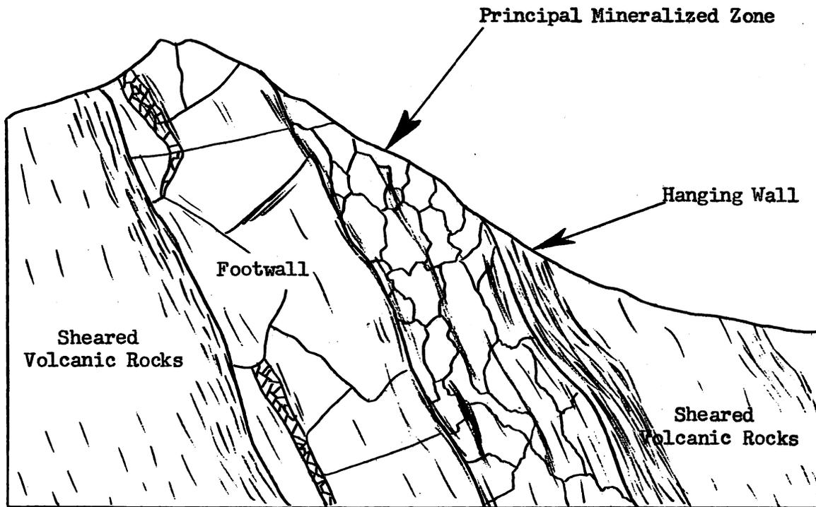
CROSS SECTION OF TYPICAL MASSIVE PYROPHYLLITE DEPOSIT
