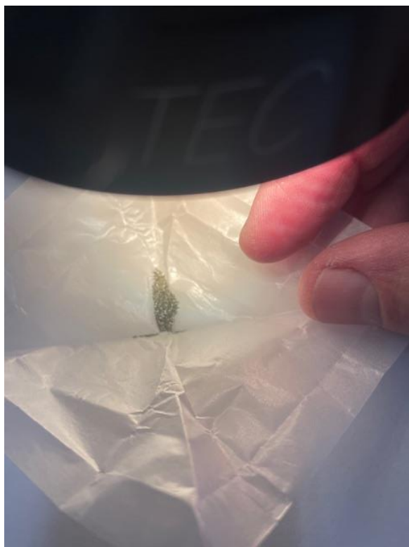
Photograph 3: Sulfides after heavy liquids and Frantz magnetic separations for Laur100K-550109. Photograph provided by Arizona LaserChron Center
