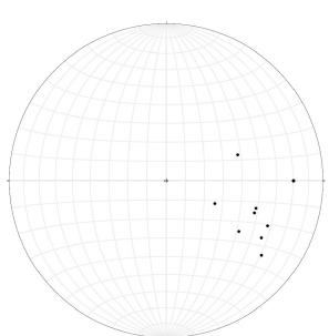
Equal Area Schmidt Net Projection of Bearing and Plunge of late phase folds axes (FL)
