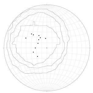
Equal Area Schmidt Net Projection of Contoured Poles to Late Phase Foliation (SL) Contour Interval = 2 sigma N =11
