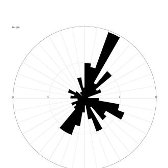
Unidirectional Rose Diagram of Joints N = 205Outer Circle = 10% Mean vector =  $013.8^{\circ} \pm 16.4^{\circ}$ Max value =15.12195% between 021° and 030°
