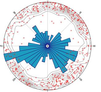
Equal area Schmidt Net projection of contoured poles to joints and unidirectional rose diagram inset. Joint count 471.
