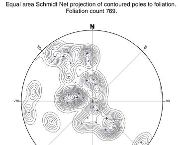
Equal area Schmidt Net projection of contoured poles to mylonitic foliation
