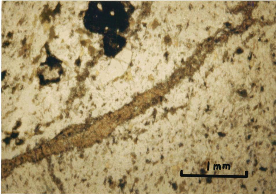
Core from a porphyritic (?) metaandesite (SC-19, 121.0')
