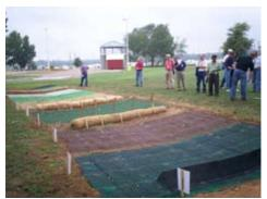
Turf reinforcement matting displayed here along with different types of diversions, including triangular silt dikes, straw wattles, and coir wattles.
