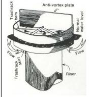
A well-designed trashrack will stop large debris that could plug the pipe but allow unrestricted passage of water and smaller debris. Some of the most effective racks allow flow to pass beneath the trash into the riser inlet as the pool level rises. Racks usually become plugged be-
