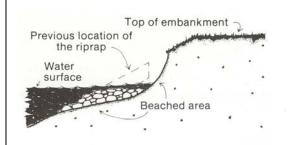
The upstream face of a dam is commonly protected against wave erosion and resultant beaching by placement of a layer of rock riprap over a layer of filter material. In some cases other materials such as steel, bituminous or concrete facing, bricks or concrete blocks are used. Beaches are sometimes constructed into small dams by placing a berm (8 to 10 feet wide) along the upstream face a few inches below normal pool. This provides a surface on which the wave energy can dissipate.
