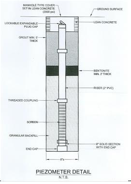
foundation soil pores and are installed at various levels in a drill hole. Readings are usually taken by measuring the elevation of water in a standpipe. Seepage pressure can be determined from piezometer readings.
