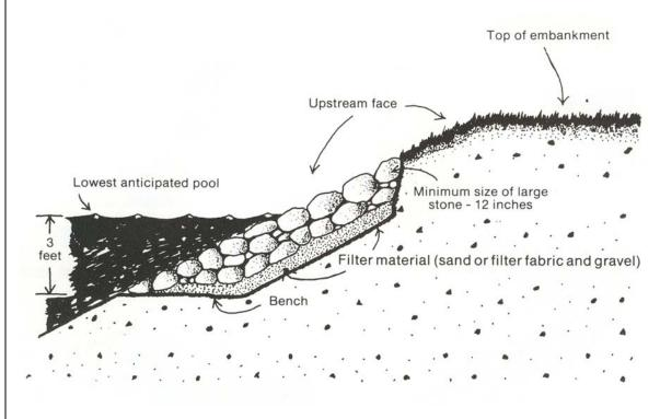
material can be washed out through these voids, and beaching develops, two filter layers will be required. The lower layer should be composed of sand or filter fabric to protect the soil surface. The upper layer should be composed of coarser materials that prevent washout through the voids in the riprap.
