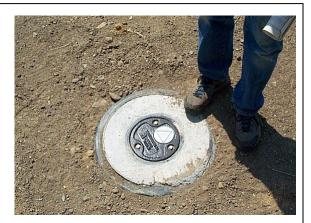
stalled in the embankment or foundation and are used to determine the ground-water level.
