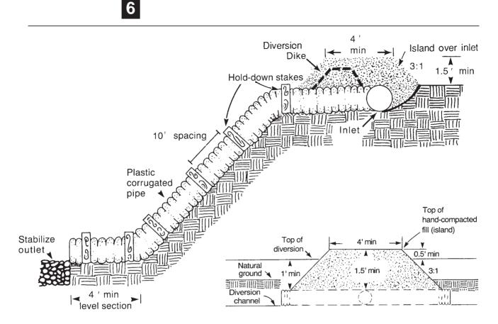
Figure 6.32a Cross section of temporary slope drain.
