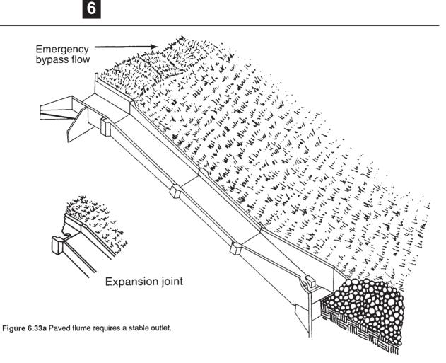
**Concrete**—Keep concrete in the flume channel at least 5 inches thick and reinforce it with 3/8-inch steel bars. Ensure that the concrete used for flumes is a dense, durable product and sufficiently plastic for thorough consolidation but stiff enough to stay in place on steep slopes. As a minimum, use a mix certified as 3,000 lb/inch<sup>2</sup>.
