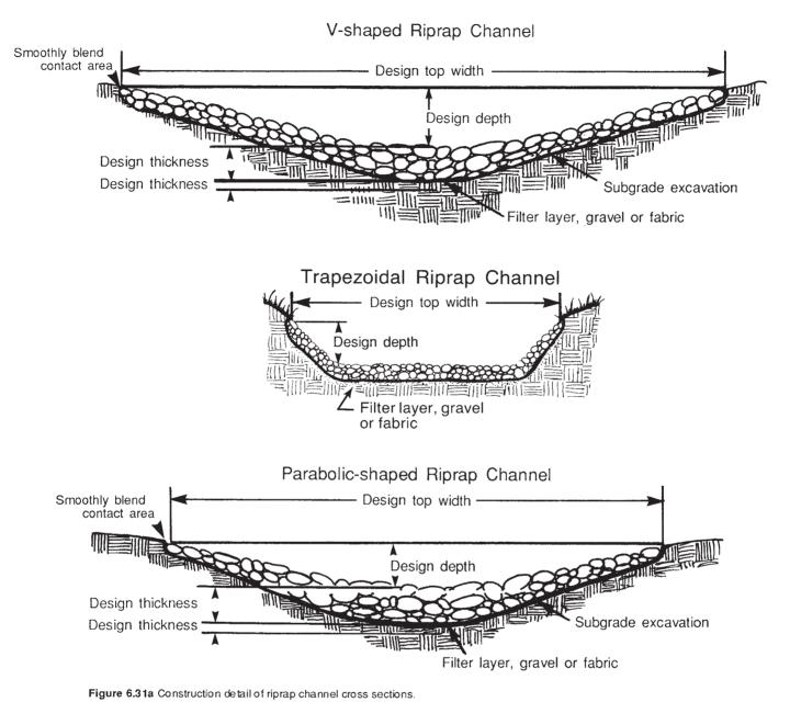
Side slope—Base side slopes on the materials and placement methods in Table 6.31b.
