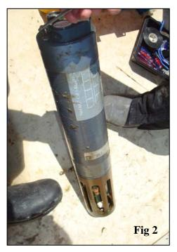
Water quality stations are equipped with a multiparameter  $YSI^{TM}$  data logger (Fig 2) sampling every 15 minutes for the following parameters: dissolved oxygen, salinity, turbidity, specific conductivity, temperature, and pH. Nutrients (ammonium, nitrate, nitrite, and ortho-phosphate) and extracted chlorophyll *a* concentrations are obtained from surface grab samples at each water quality station monthly.
