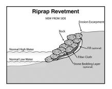
**REVETMENTS** are sloped structures built against the shoreline to absorb wave energy and prevent erosion. Building materials include rock, concrete and oyster shells. These structures are long lasting and can be combined with marsh grass plantings. The riprap provides habitat for some aquatic species. Revetments should be placed as far landward as possible to conserve the intertidal zone.
