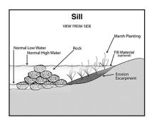
**SILLS** made of rock or oyster shells are placed just off the shoreline to break up wave energy. This allows vegetation to take root. The sill may provide habitat for aquatic organisms like algae, shellfish, crustaceans and fish. Sediment can be added behind the sill and planted with cordgrass, a native marsh plant. The top of the sill usually extends just above the high water mark.
