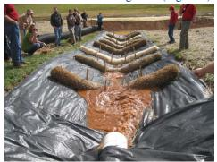
Figure 1. Wattles installed with PAM.
