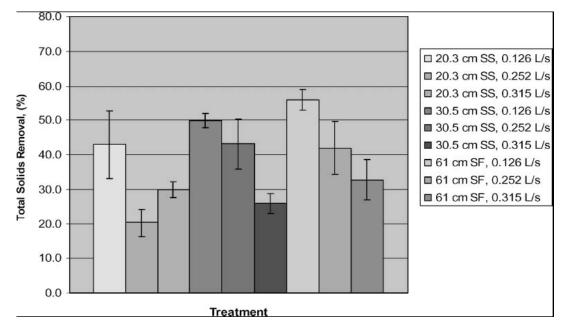
**Figure 1.** Total solids removal efficiency for diam 8 in (20.3cm) coarse SiltSoxx (SS), 12 in (30.5cm diam) coarse SiltSoxx, and 24 in (61cm) silt fence (SF) with a height of 18" (45.7 cm) above the flume, with corresponding flow rates. The standard error of the means for each treatment is shown. Flow rates tested were 2, 4, and 5 gpm (0.126, 0.252, and 0.315 L/s) (Keener et al, 2007).
