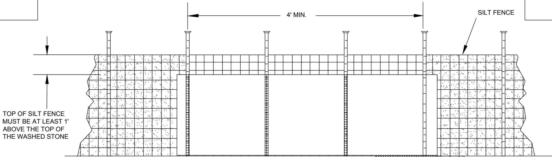
TOP OF SILT FENCE MUST BE AT LEAST 1' ABOVE THE TOP OF THE WASHED STONE
