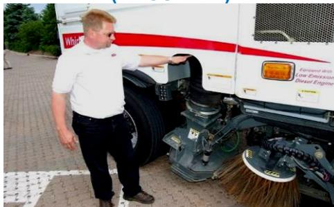
Vacuum street cleaners are the least common and most expensive. They apply a strong vacuum to a relatively narrow area that lifts particles both at and below the surface of the pavement. Vacuum sweepers have demonstrated their ability to suction 3 to 4 inches of gravel from PICP and can restore infiltration to some types of pavements that have been grossly neglected. (Hunt, NCSU-BAE)
