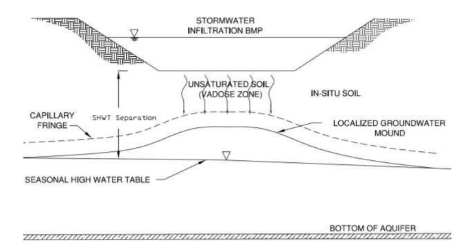
Snapshot of groundwater interaction with an infiltration BMP during a drainage event. Mounding can occur locally, which reduces the drainage gradient of water in the BMP.
