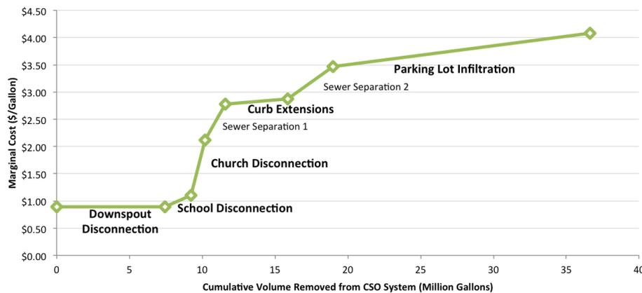
**Figure 2.** Costs and Cumulative Volume of Stormwater Removed from the CSO System through Various Grey and Green Strategies (Green in Bold). Source: ECONorthwest, with data from City of Portland 2005
