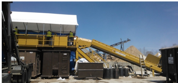
The raised picking line shown above allows workers to sort a variety of materials, including cardboard, wood, masonry, metal, plastic bottles and paper, for recycling.
