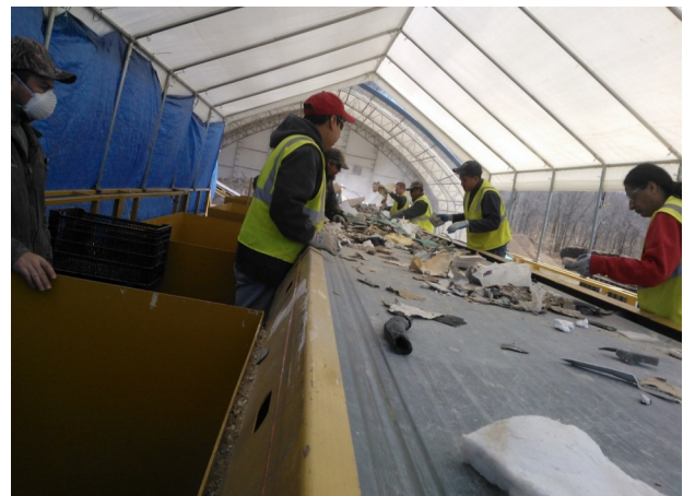
Todco's crew of temporary employees sort mixed construction debris for recycling as it moves past on the picking line's conveyor belt.
