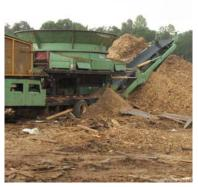
A tub grinder is used to process clean wood waste into boiler fuel.
