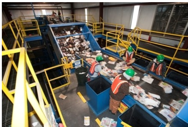
Workers sort materials prior to further processing by a newspaper sorting screen.
