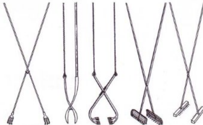
Figure 8. An illustration of several different designs for hand tongs and rakes that may be used for harvesting oysters. From Shafi 2007, reproduced from von Brandt 1964.
