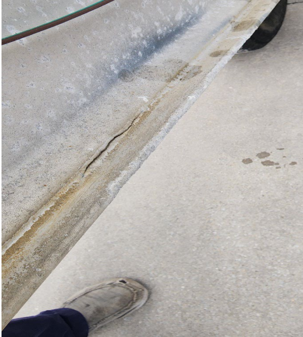
Cracks along main trailer frame
