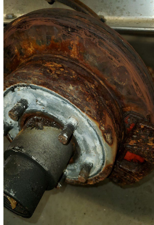
Rusted brake rotor
