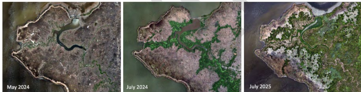
Fig. 8: Wetland vegetation growth (2024-2025) following thin layer placement at Deal Island Wildlife Management Area. Image courtesy of Dr. Jenny Davis, NOAA (Appendix B).
