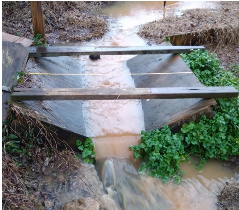
Figure 9. Trapezoidal flume for NT monitoring station.
