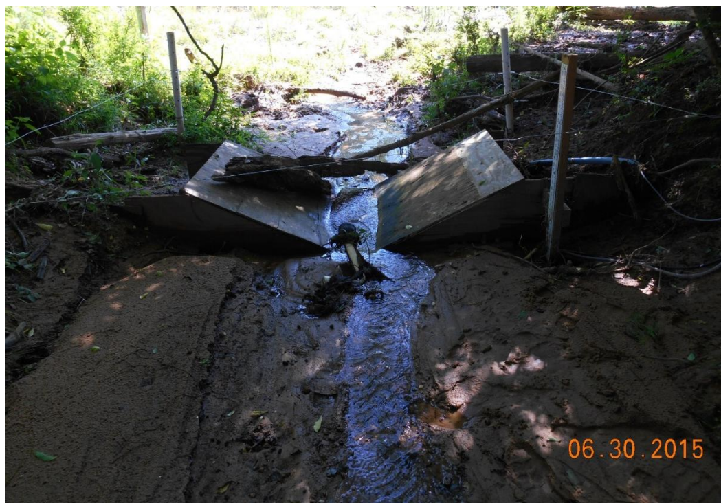
Figure 17. Picture of UTA stream flume and sediment deposition on 6/30/15.
