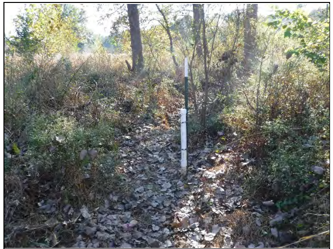
Flow Gauge in Reach UT4-R2 (photo 11/6/19)
