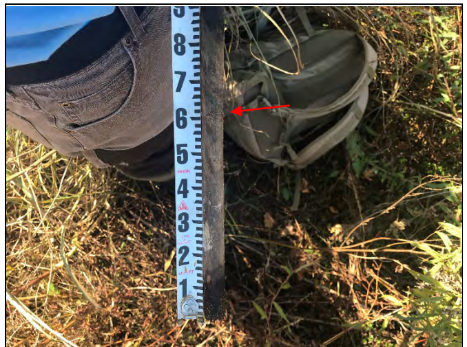
Crest Gauge Reach HC-R1: Overbank event of 0.60' (photo from 8/8/19)
