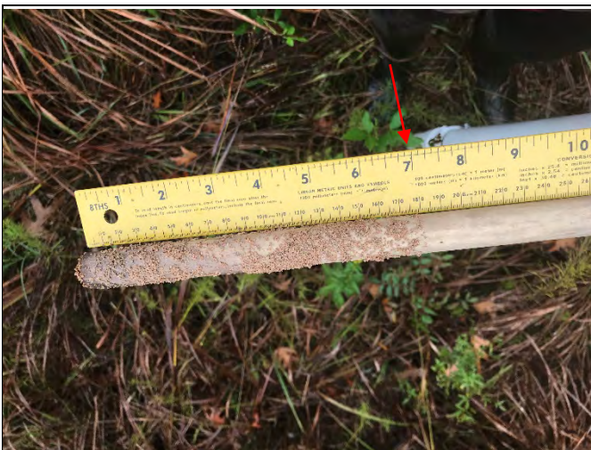
Crest Gauge Reach UT4-R2: Overbank event of 0.58' (photo from 10/16/19)
