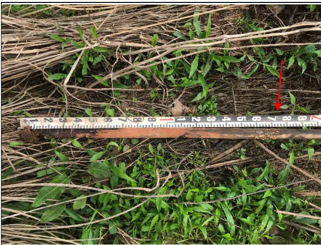
Crest Gauge Reach HC-R1: Overbank event of 1.72' (photo from 4/12/19)
