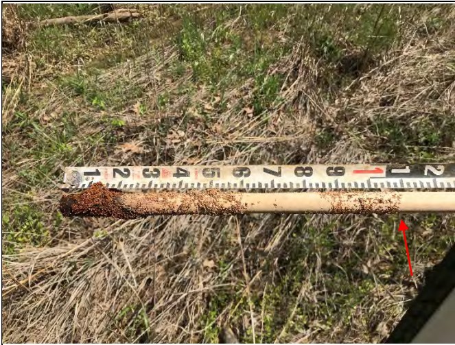
Crest Gauge Reach UT4-R2: Overbank event of 1.09' (photo from 4/11/19)
